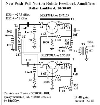
base amplifier (this change due to Rohde). Different input transformer turns ratios (and, presumably, different transistor transformer turns ratios as well as different output turns ratios) provide different gains and different intercepts. Rohde's article contains formulas which may be useful to estimating turns ratios, but they were beyond me. I used trial and error to arrive at the turns ratios for my amplifiers.
