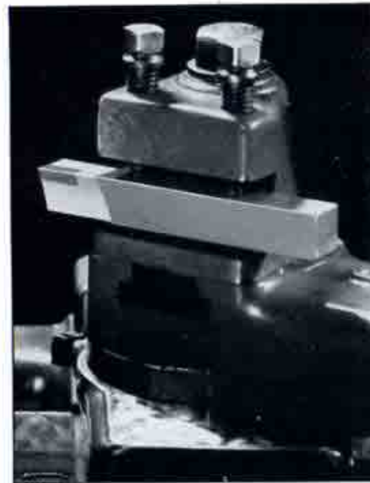
Fig. 50. Tungsten Carbide Tipped Cutting Tool Mounted in Open Side Tool Post for Rigid Support.
