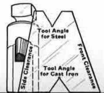
Fig. 23. Checking side clearance of cutter bit.
