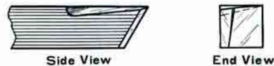
Fig. 27. Detail of roughing tool.
