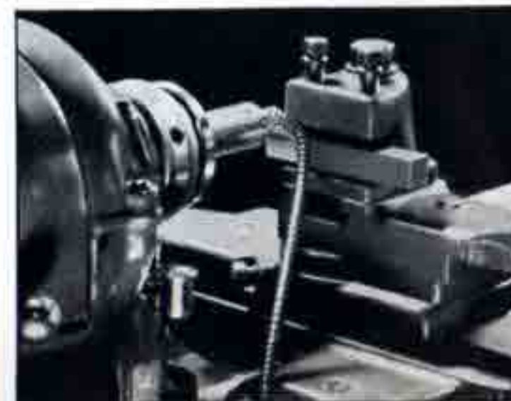
Fig. 51. Machining a Steel Shaft at High Speed with Tantalum Carbide Tipped Cutting Tool.
