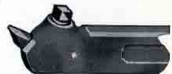
Fig. 5. Cutter bit inserted in tool holder ready to use.
