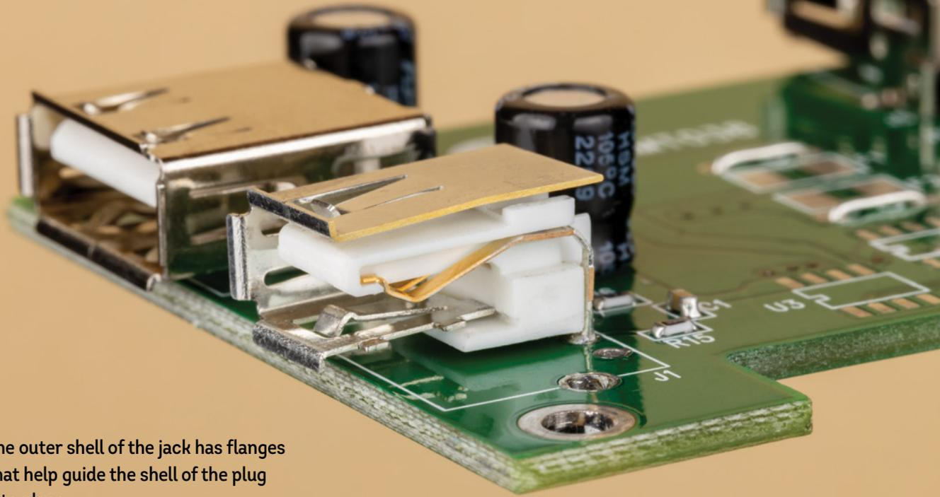
The outer shell of the jack has flanges that help guide the shell of the plug into place.
