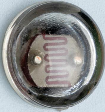
Photoresistors are used in circuits that sense light but don't require fast response times, including night-lights, streetlamps, and auto-darkening mirrors.
