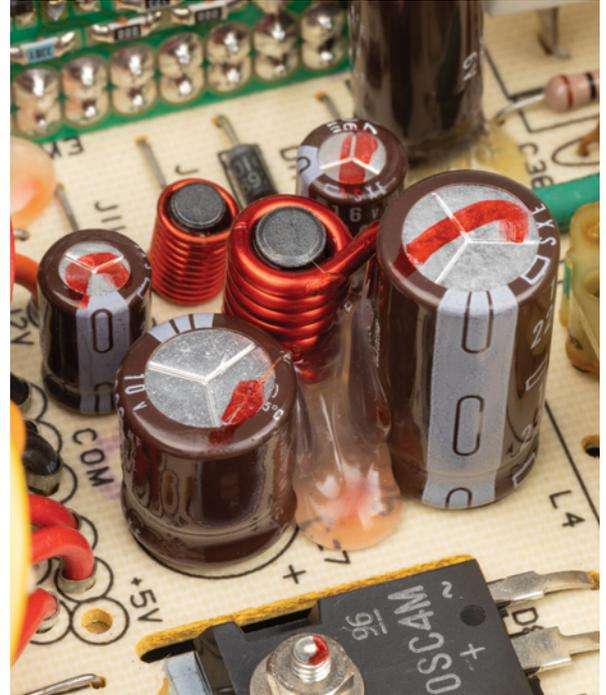
Before it's anodized, the aluminum foil is etched in such a way as to substantially increase its surface area, and thus its capacitance.
