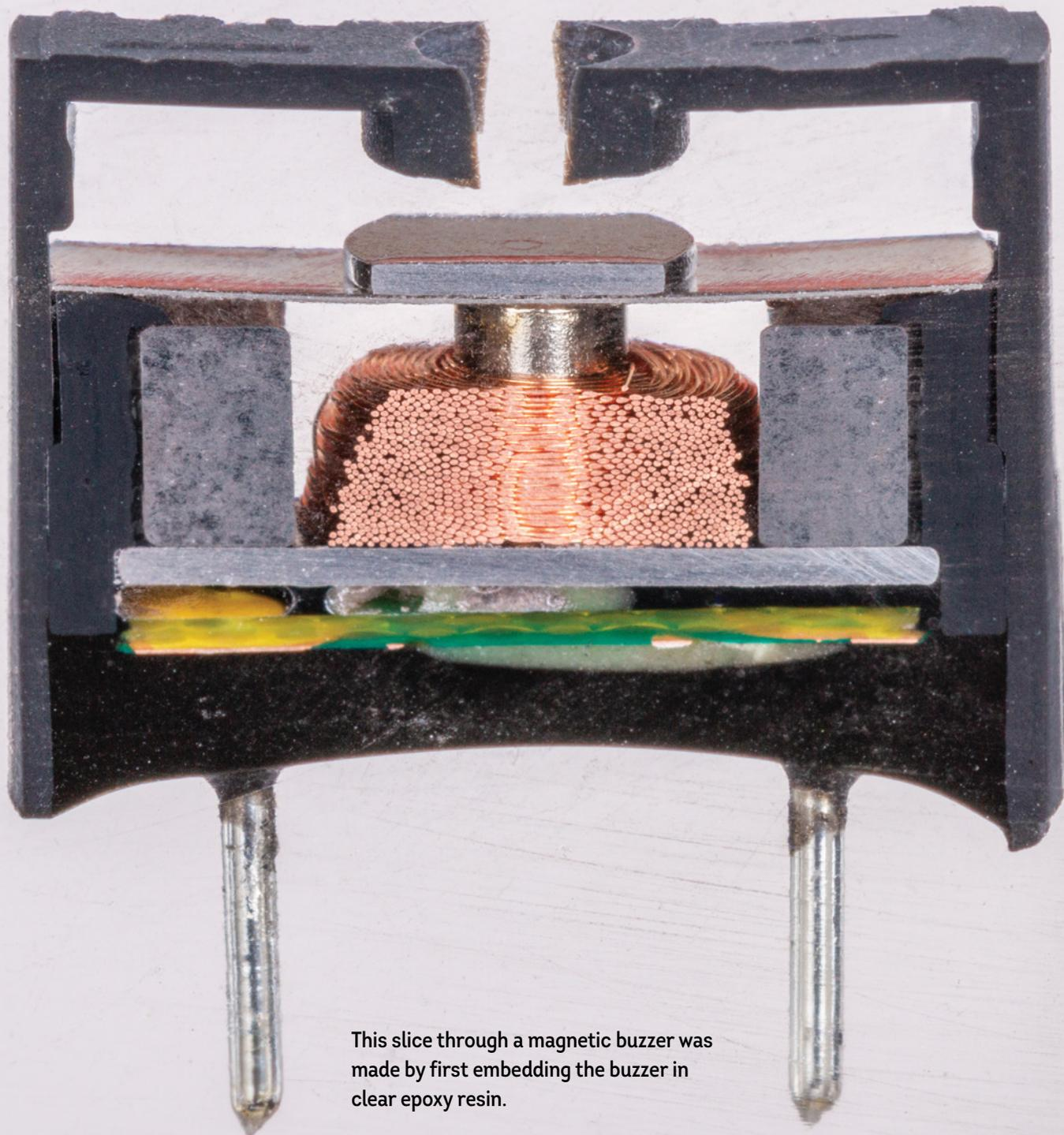
This slice through a magnetic buzzer was made by first embedding the buzzer in clear epoxy resin.
