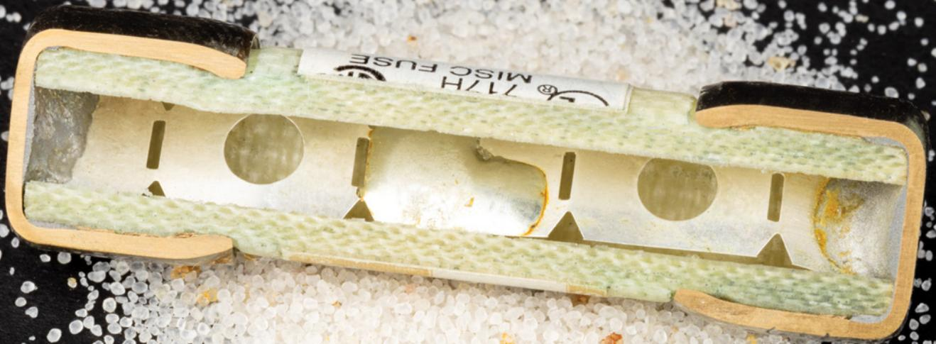
Like the fluid in a liquid power fuse, the sand inside this fuse prevents arcing.
