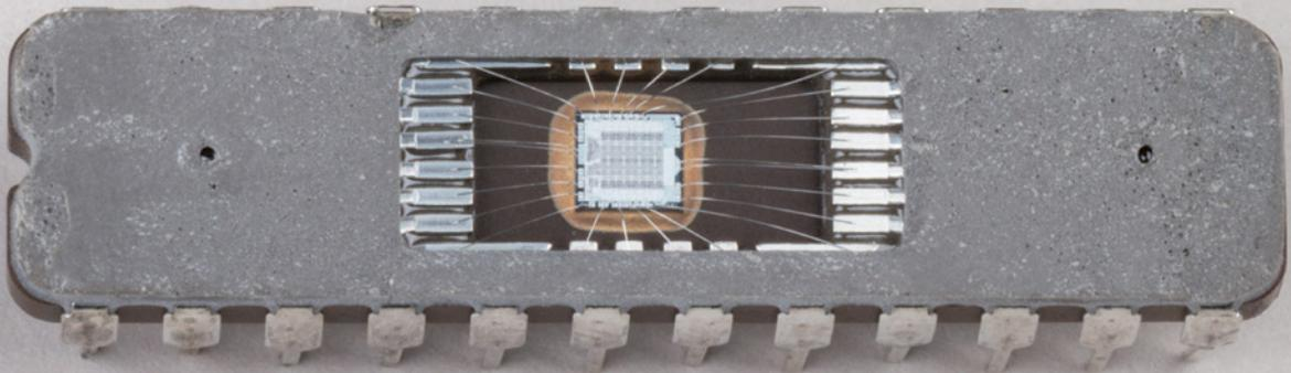
Each active pin on the package is paired with at least one bond wire that connects to the IC within.
