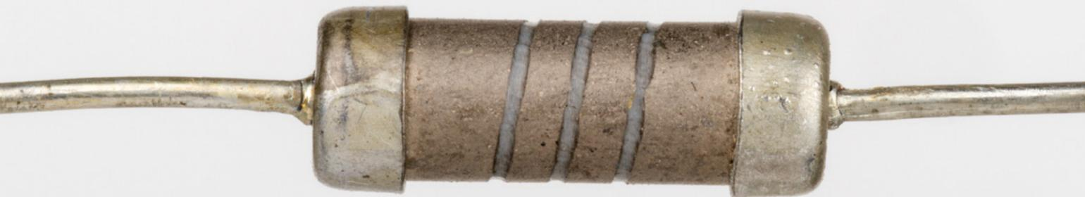
The spiral groove can clearly be seen after the protective coating has been removed.
