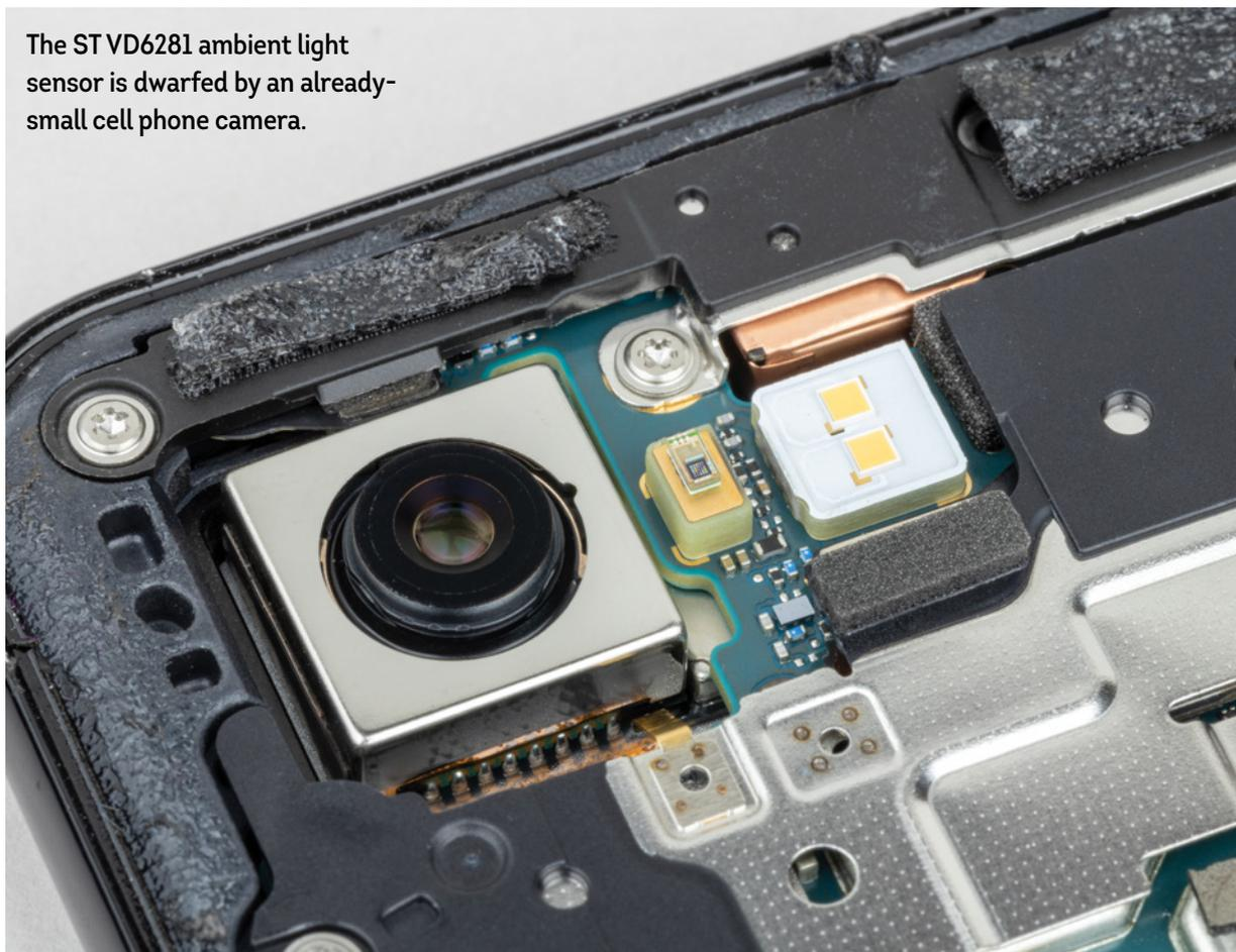
The sensor sits on a circuit board riser that raises it to about the same height as the flash on the back surface of the phone. This gives the sensor the widest possible field of view.
