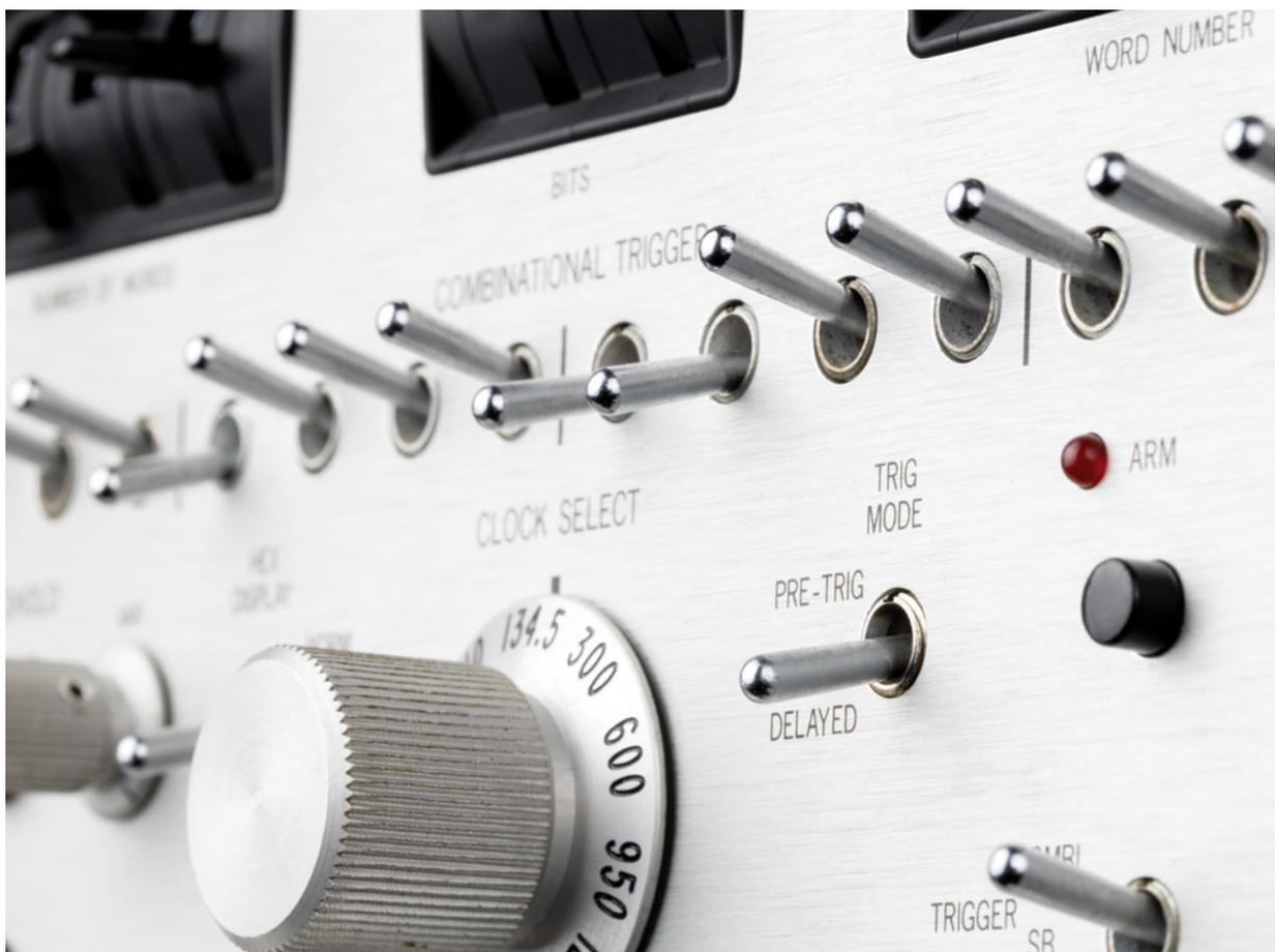
The upper section of the switch is threaded for mounting to a panel. The pin through the threaded section is the pivot point for the lever.
