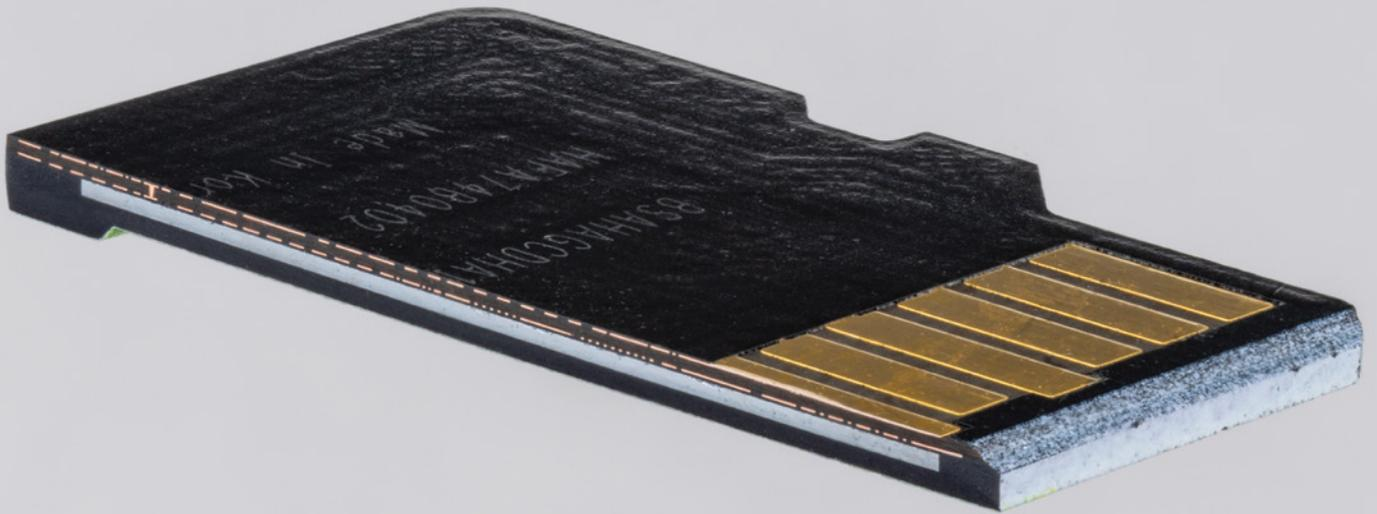
The entire back surface of the microSD card is a two-layer circuit board. The large contact fingers are simply exposed copper areas from the upper layer of the PCB, with a gold-plated finish.
