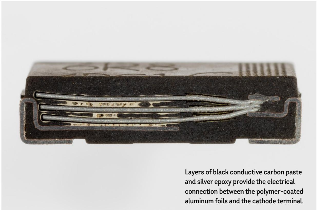
Layers of black conductive carbon paste and silver epoxy provide the electrical connection between the polymer-coated aluminum foils and the cathode terminal.
