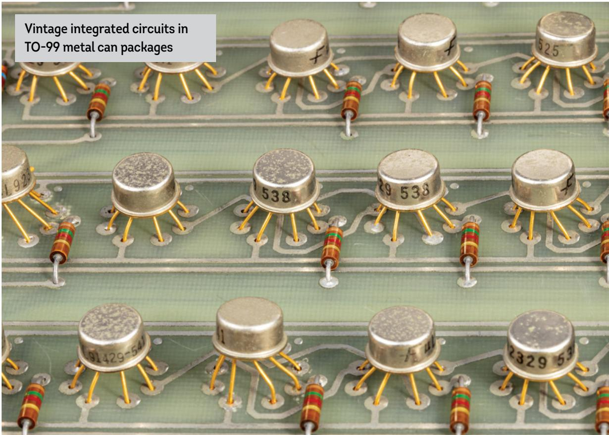
The chip is connected through eight bond wires. Seven go to pins insulated with glass seals. The eighth pin is electrically connected to the can.
