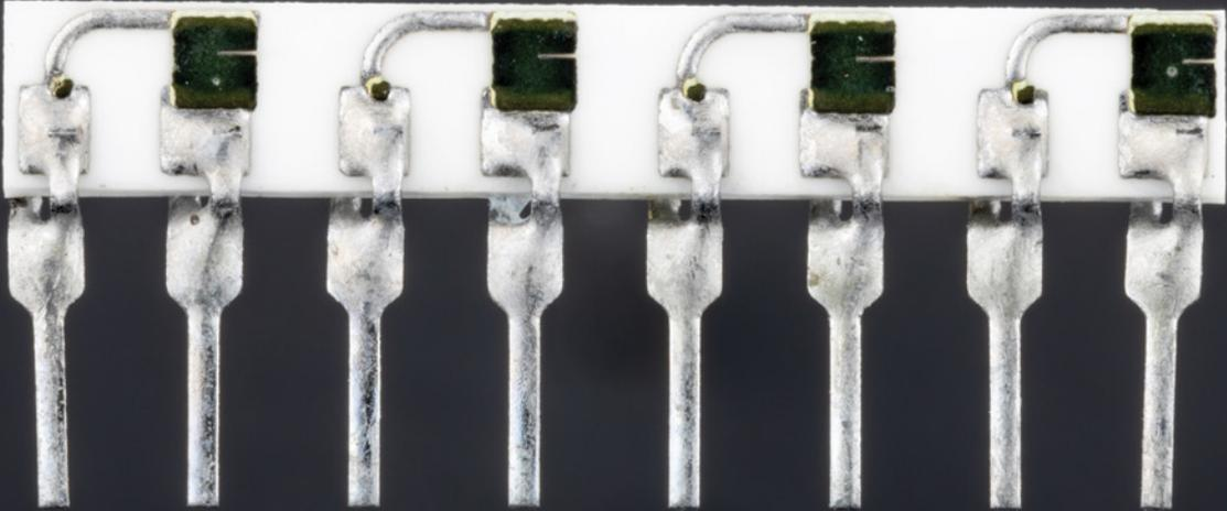
Straight cuts in the greenish resistive material mark the path of the trimming laser.
