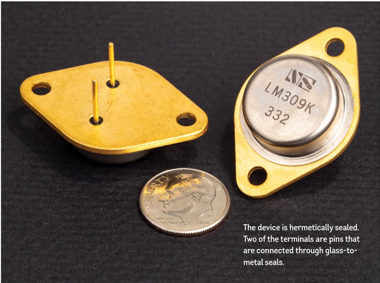
The device is hermetically sealed. Two of the terminals are pins that are connected through glass-to-metal seals.
