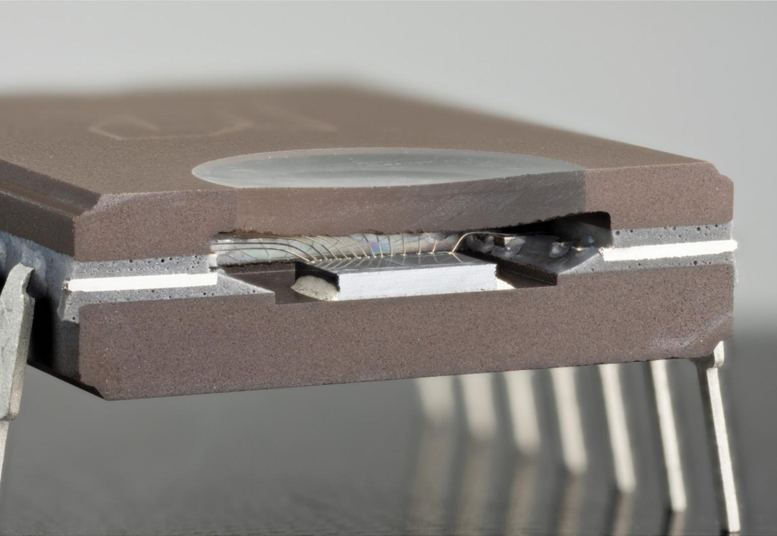
The ceramic DIP of an EPROM has a quartz-glass window that allows ultraviolet light to erase the memory on the silicon die.
