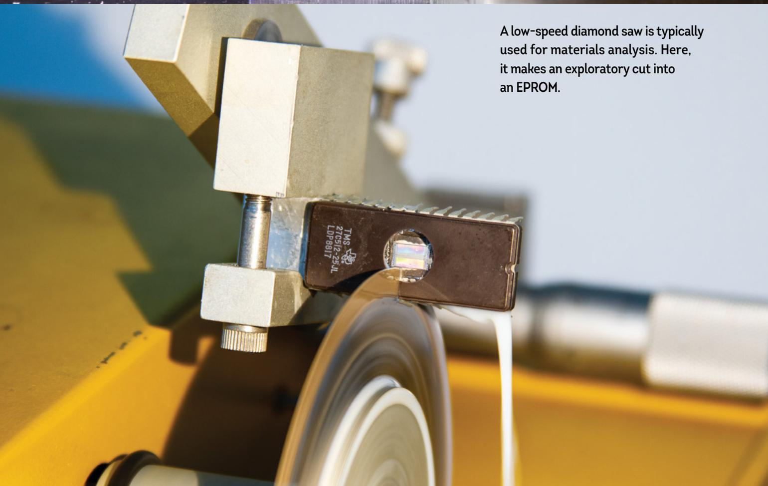
A low-speed diamond saw is typically used for materials analysis. Here, it makes an exploratory cut into an EPROM.
