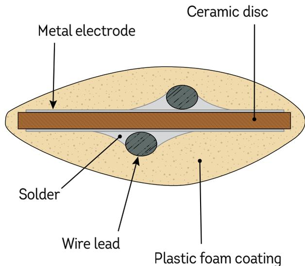
The metal layers on the surfaces of the ceramic disc are so thin that it can be hard to see them in cross section.
