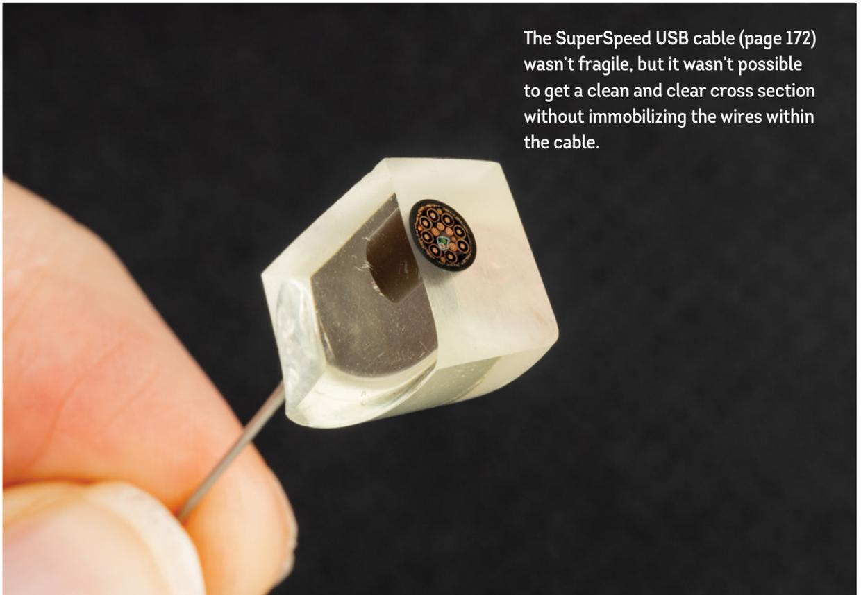
The SuperSpeed USB cable (page 172) wasn't fragile, but it wasn't possible to get a clean and clear cross section without immobilizing the wires within the cable.
