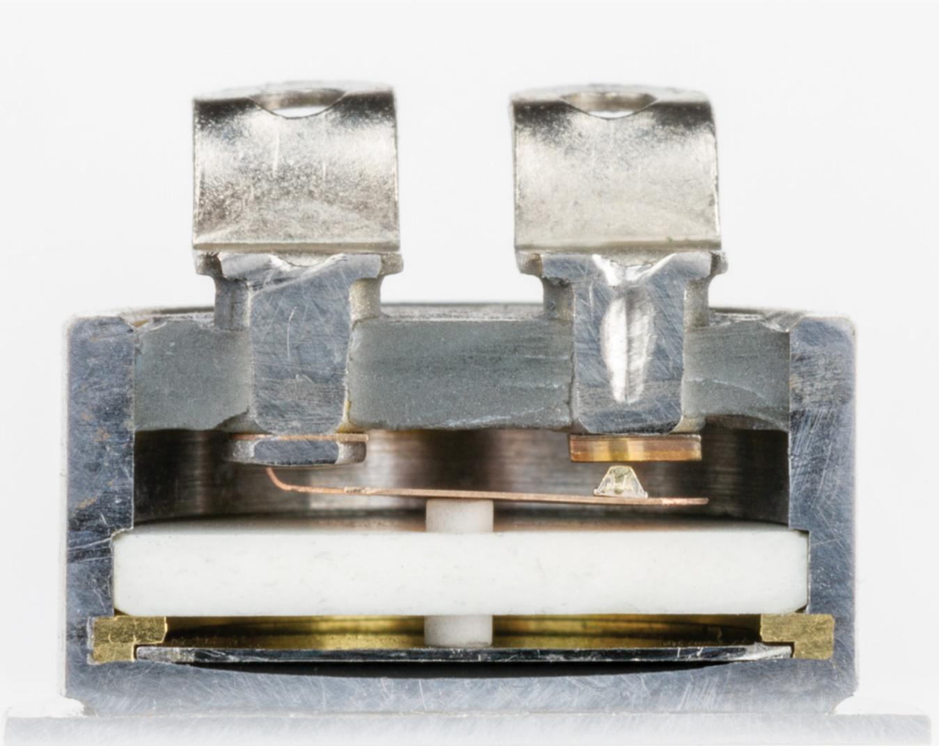
This thermal switch has been cut in half to show its mechanism. Normally, a switch like this is sealed to prevent dust from getting inside.
