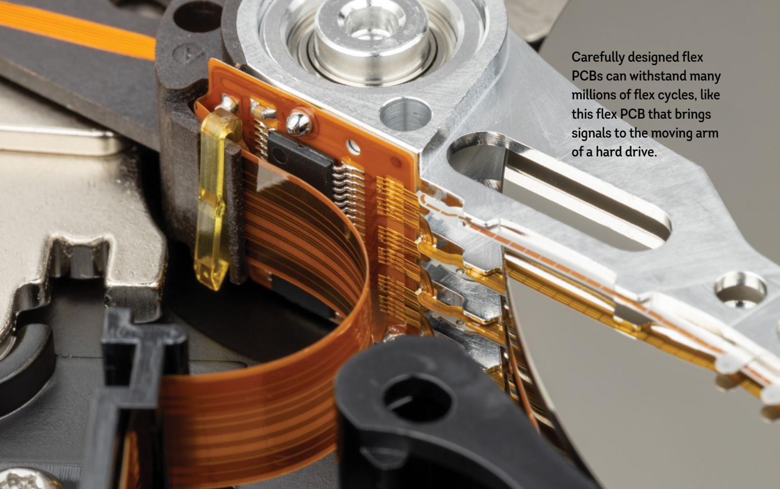
Carefully designed flex PCBs can withstand many millions of flex cycles, like this flex PCB that brings signals to the moving arm of a hard drive.
