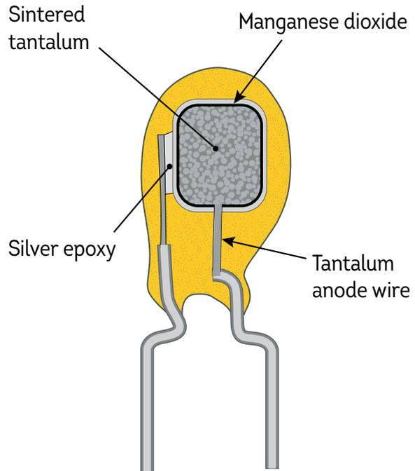
Connecting a tantalum capacitor backward causes chemical changes that damage the thin oxide layer. The label on the dipped plastic coating indicates the anode lead with “++.”
