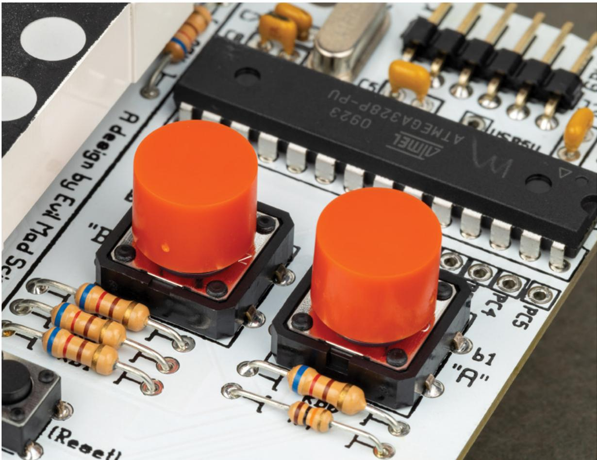
This tactile switch has a large red button cap. Low-profile versions are ubiquitous in electronics.
