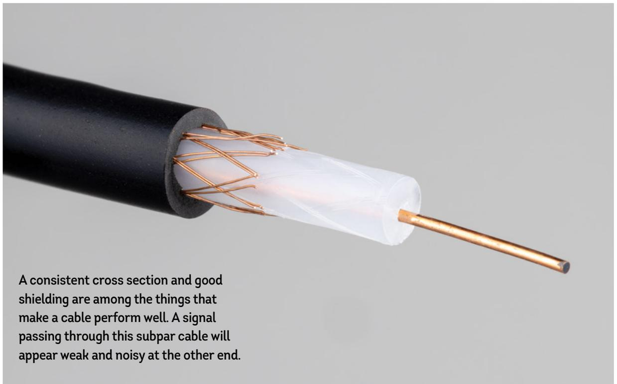
A consistent cross section and good shielding are among the things that make a cable perform well. A signal passing through this subpar cable will appear weak and noisy at the other end.
