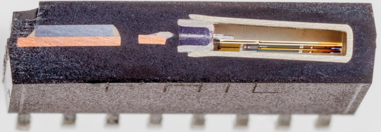
The gray integrated circuit die can be seen on the left, atop the copper lead frame, leaving room for the 32 kHz quartz crystal on the right.
