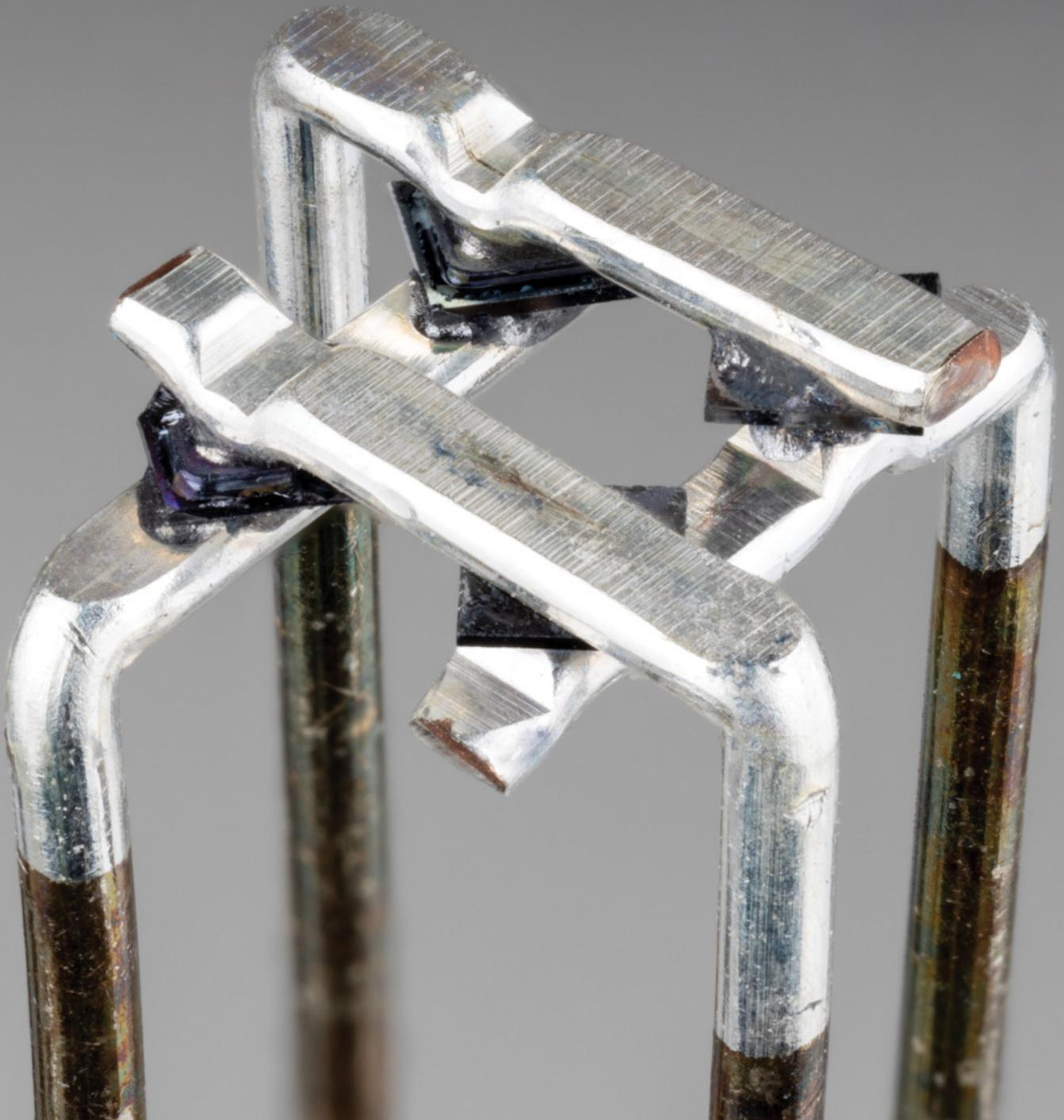
The wire leads are silver-plated copper. Their lower parts were tarnished by exposure to the air; the crisp, clean silver part was protected by the plastic package.
