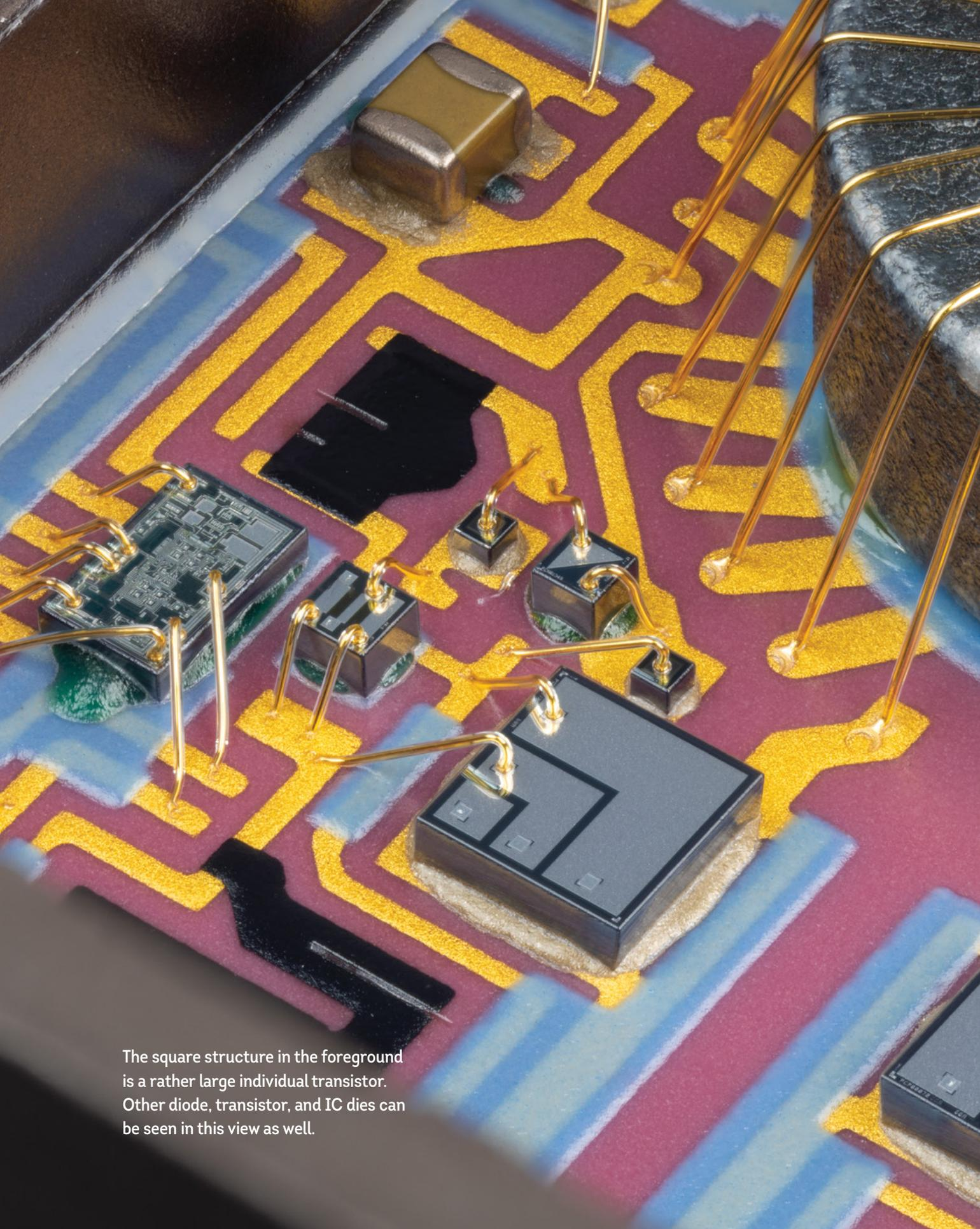
The square structure in the foreground is a rather large individual transistor. Other diode, transistor, and IC dies can be seen in this view as well.
