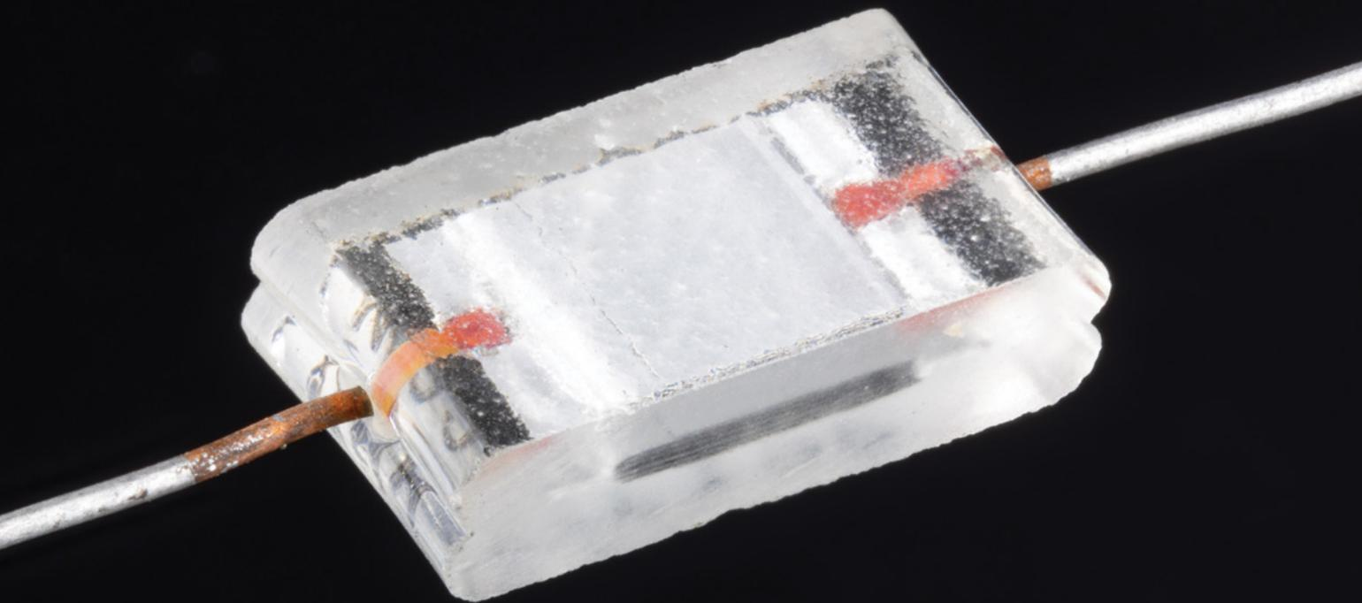
For robustness, the same type of glass used between the foil layers is also used as the outer packaging of the device, about 5 mm thick.
