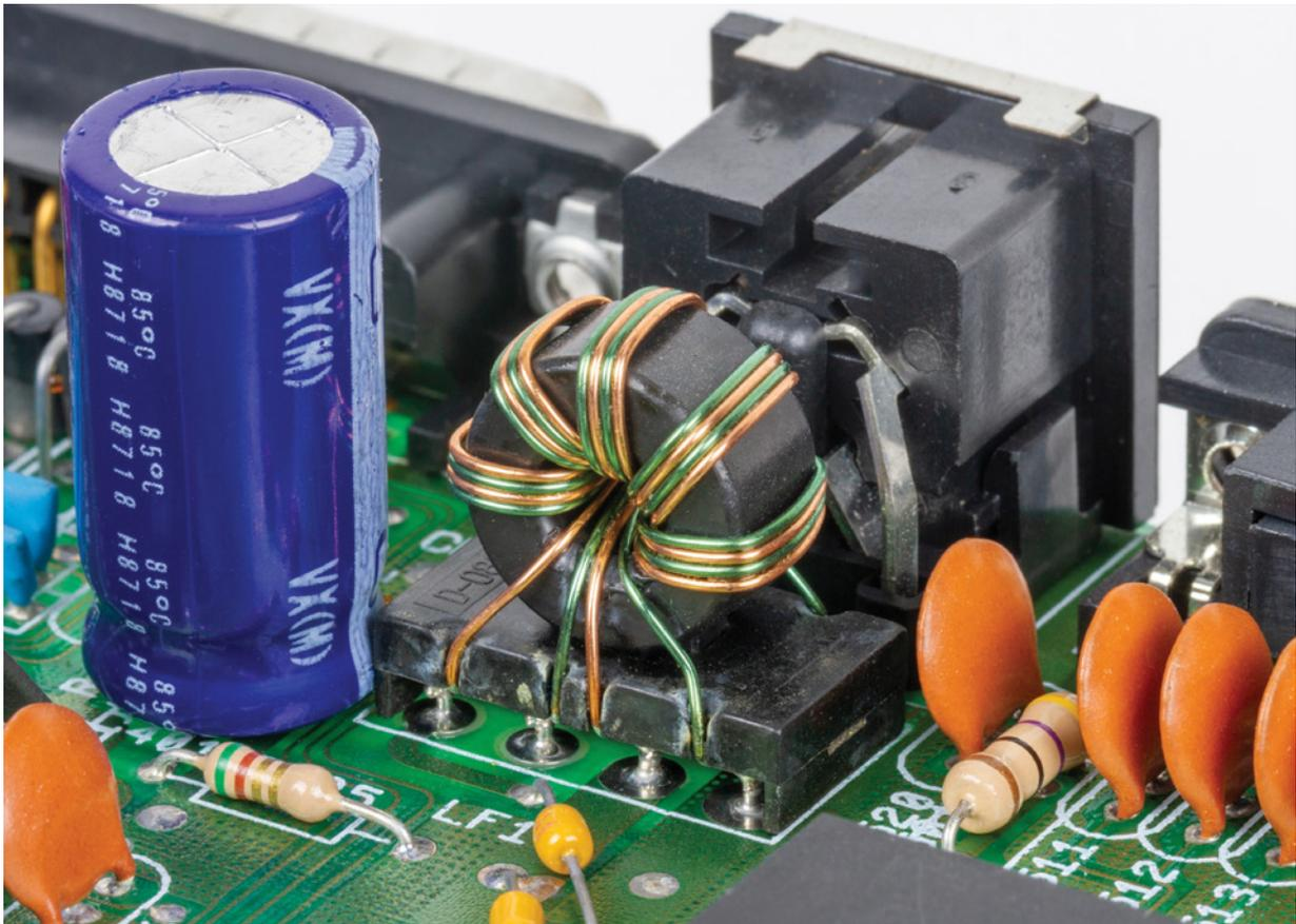
This transformer is configured as a choke: a special type of transformer designed to stop stray radio waves from leaking outside of a piece of electronics.
