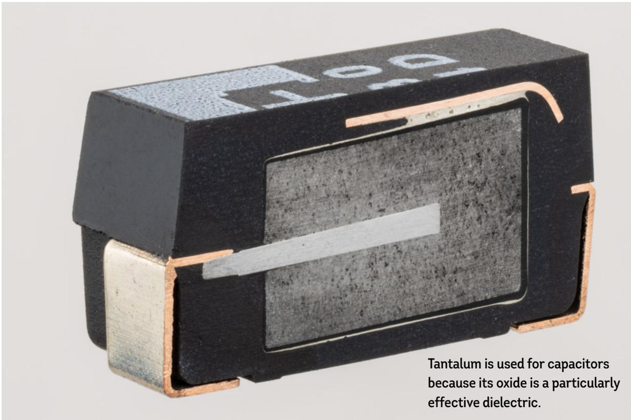
Tantalum is used for capacitors because its oxide is a particularly effective dielectric.
