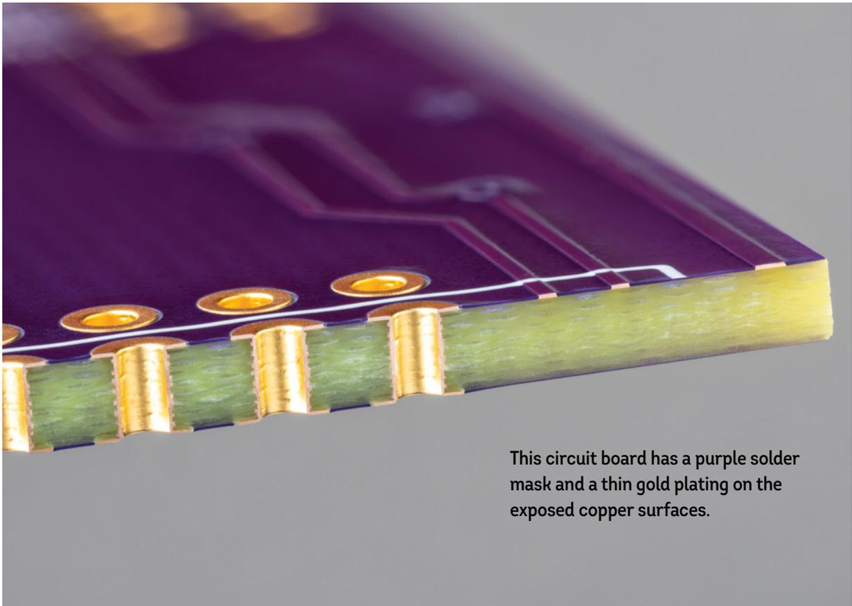
This circuit board has a purple solder mask and a thin gold plating on the exposed copper surfaces.
