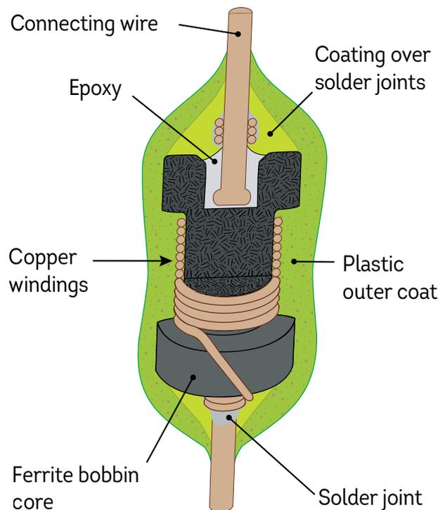
The copper leads are attached to the ferrite ceramic core with beige epoxy prior to winding the copper wire.
