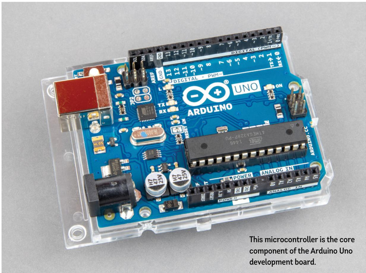
This microcontroller is the core component of the Arduino Uno development board.
