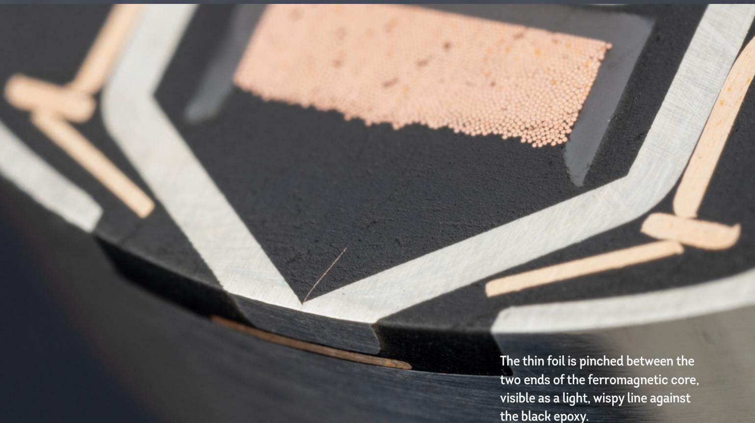
The thin foil is pinched between the two ends of the ferromagnetic core, visible as a light, wispy line against the black epoxy.
