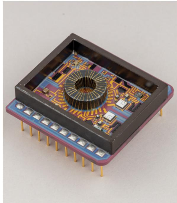
There are no electrical connections between the left and right halves of this amplifier module. The left side is the input side, and the right is the output.
