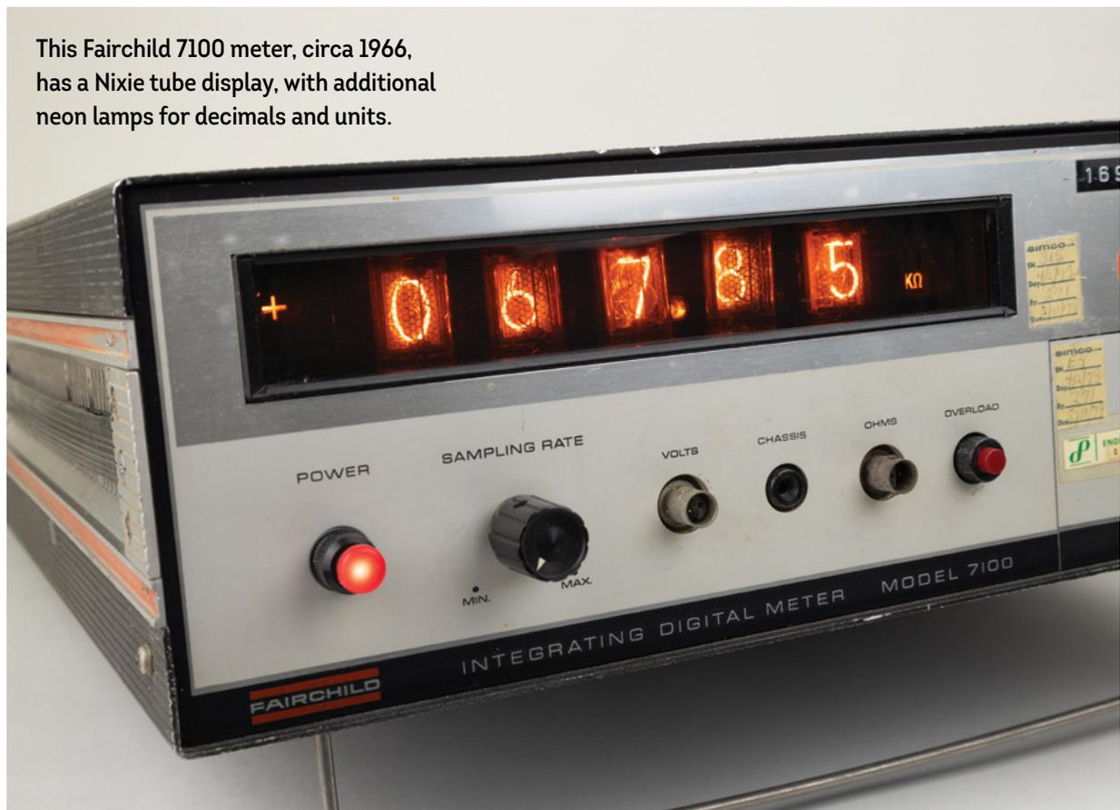
A ZM1030 Nixie tube has an orange coating to increase the display contrast.
