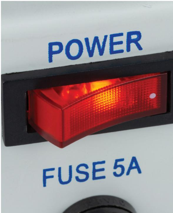
Neon lamps are often used as indicators for AC power—for example, in extension cords, light switches, and power switches.
