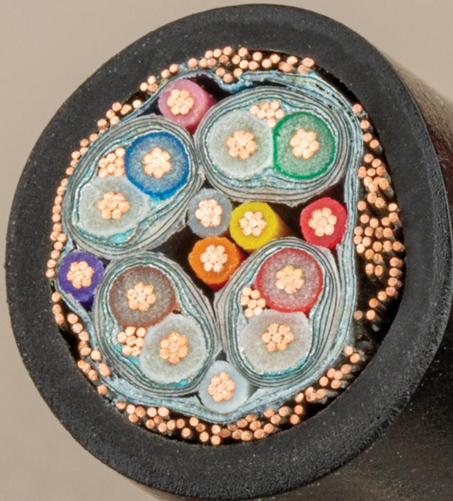
Each signal pair is shielded with a foil wrap and copper drain wire.
