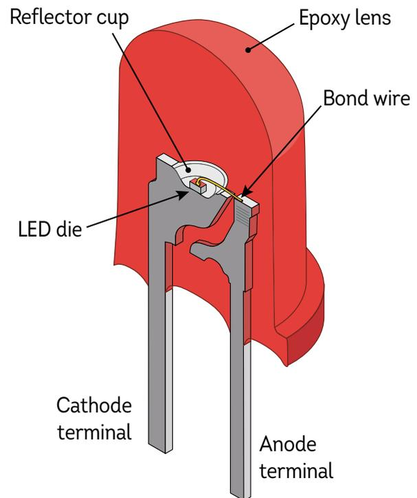
LEDs are planar devices: only the top surface of the semiconductor die emits light. The dies are cut into neat cubes for ease of handling.
