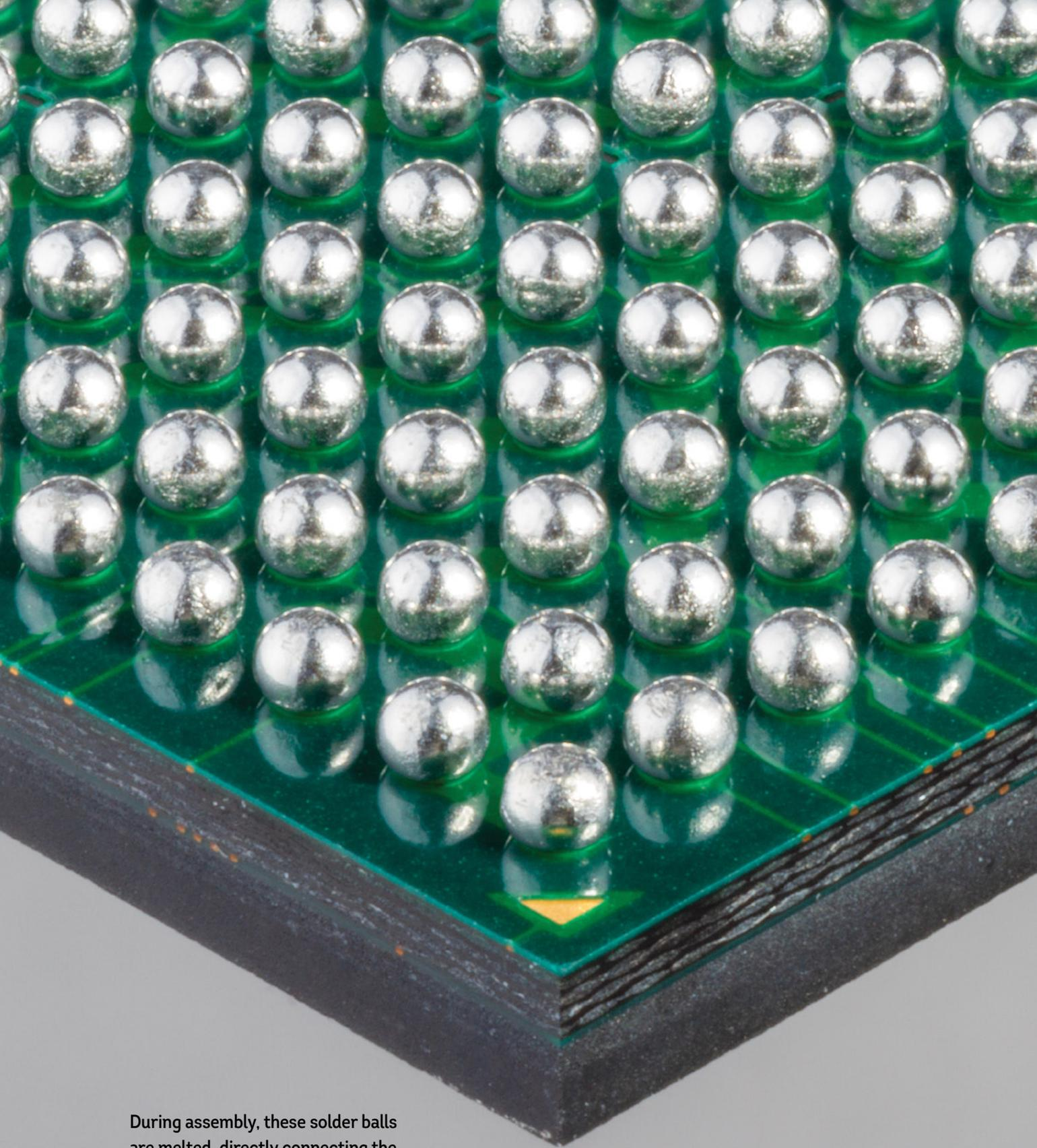
During assembly, these solder balls are melted, directly connecting the component to the circuit board at many points—sometimes thousands.
