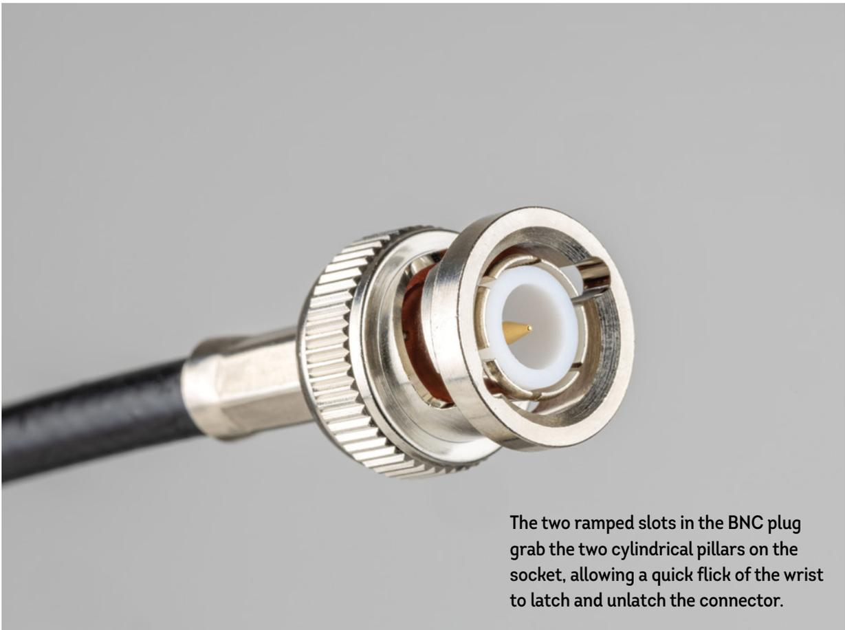
The two ramped slots in the BNC plug grab the two cylindrical pillars on the socket, allowing a quick flick of the wrist to latch and unlatch the connector.
