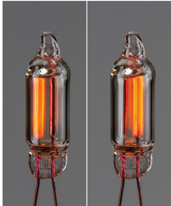
At any given instant, only one electrode is actually lit. Because they alternate quickly, it looks as though both are lit.
