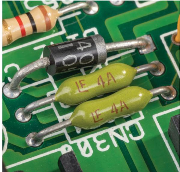
This fuse has a thin wire, bent in a pattern to keep it in a consistent shape with consistent thermal properties.
