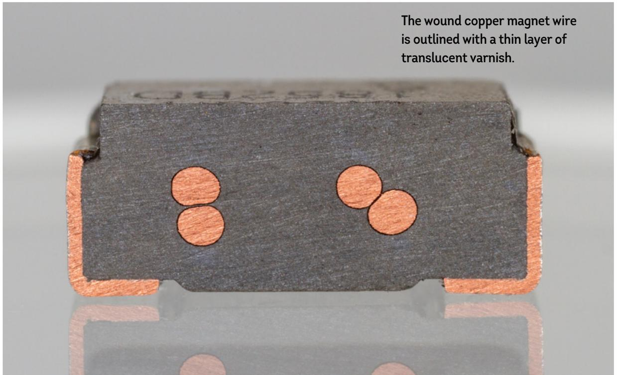
The wound copper magnet wire is outlined with a thin layer of translucent varnish.
