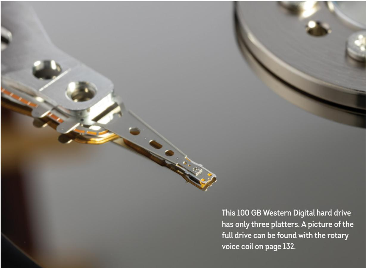
This 100 GB Western Digital hard drive has only three platters. A picture of the full drive can be found with the rotary voice coil on page 132.
