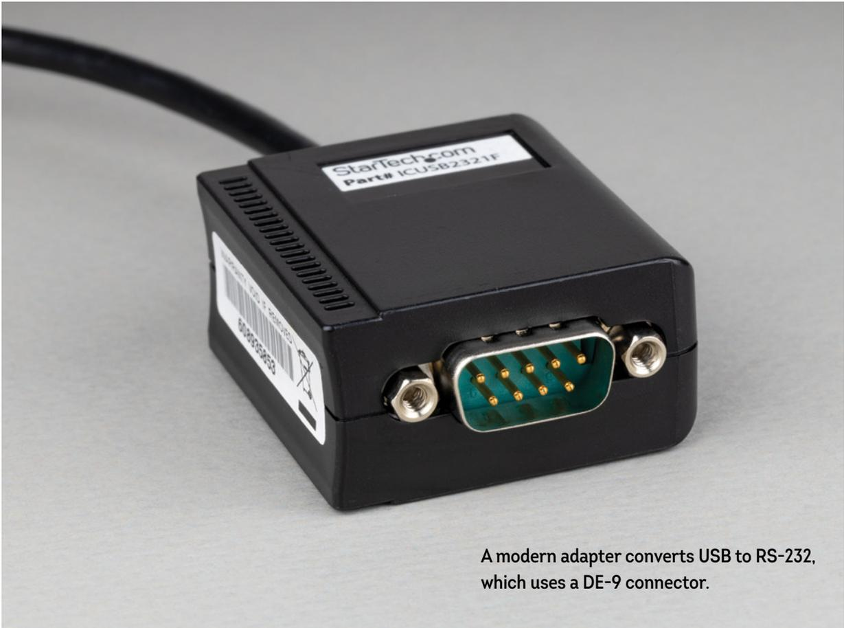
A modern adapter converts USB to RS-232, which uses a DE-9 connector.
