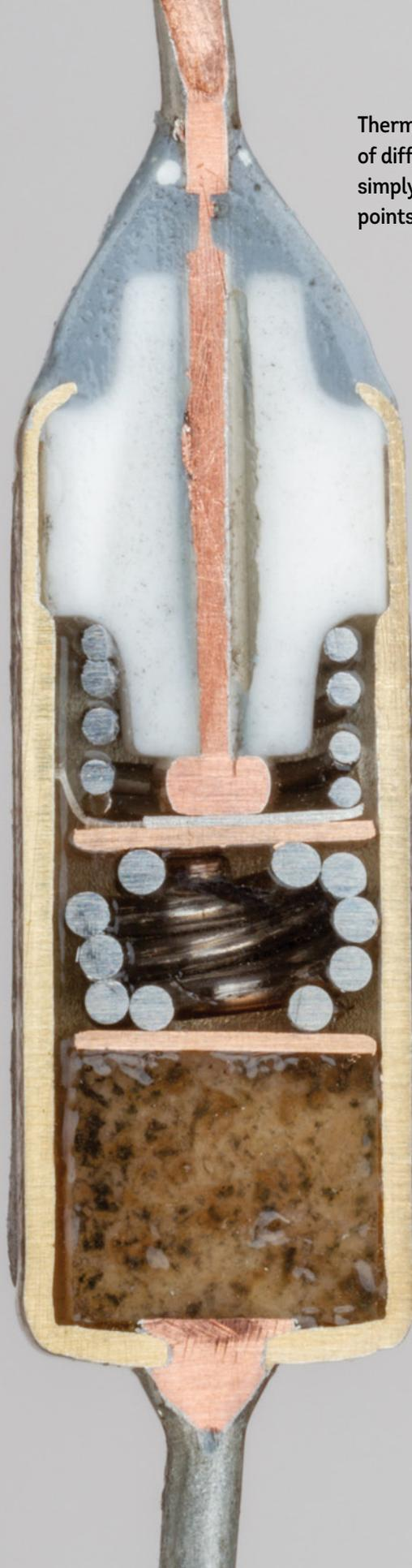
Thermal fuses are available with a range of different temperature ratings, which simply represent different melting points of the wax.
