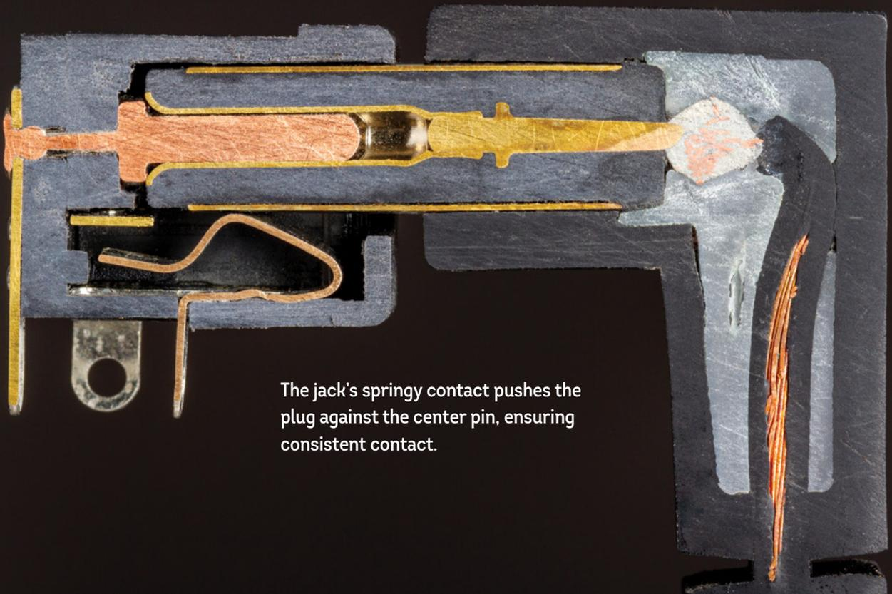
The jack's springy contact pushes the plug against the center pin, ensuring consistent contact.
