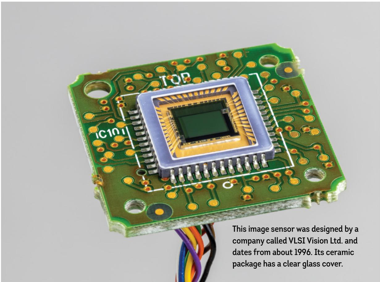
This image sensor was designed by a company called VLSI Vision Ltd. and dates from about 1996. Its ceramic package has a clear glass cover.
