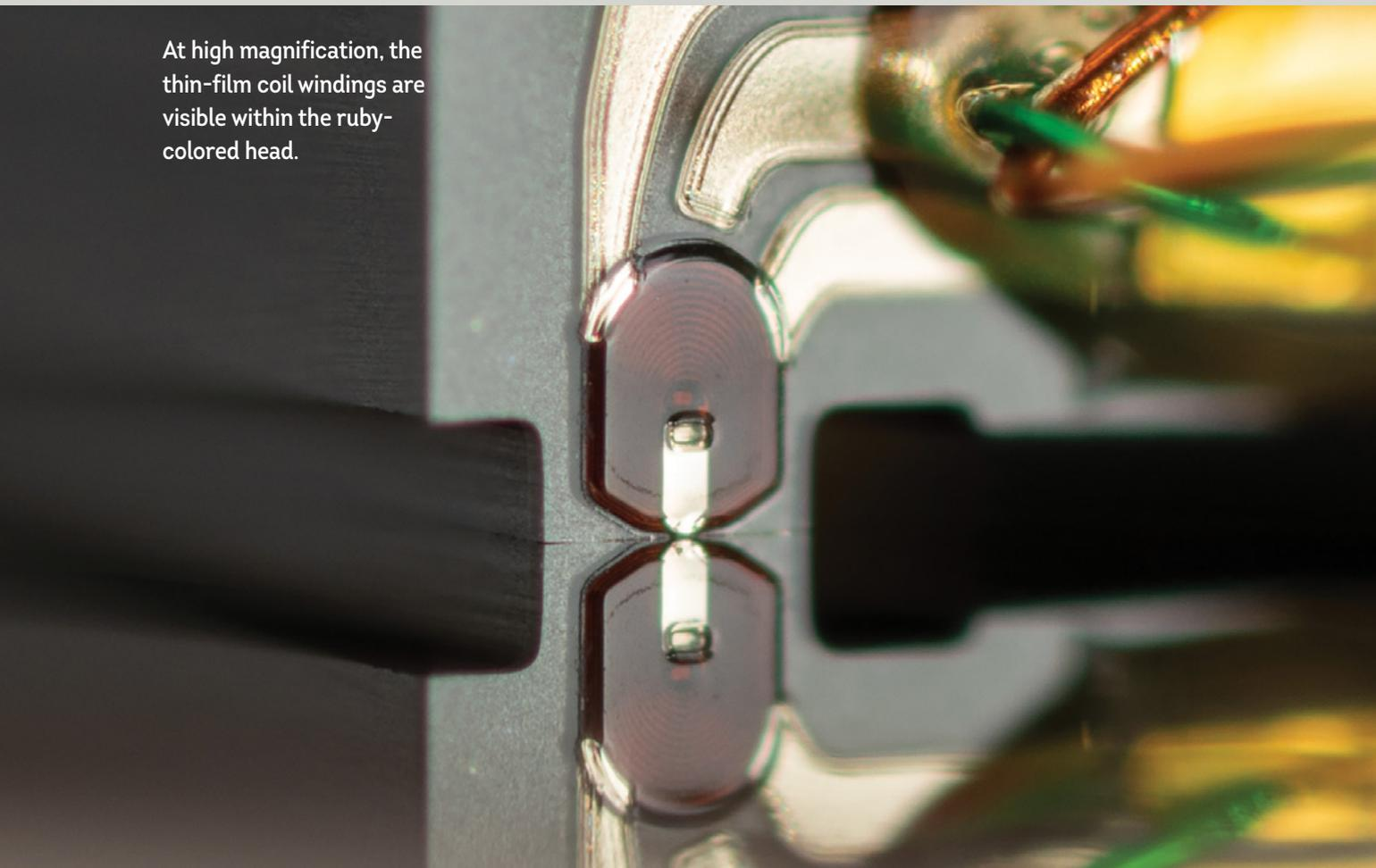
At high magnification, the thin-film coil windings are visible within the ruby-colored head.
