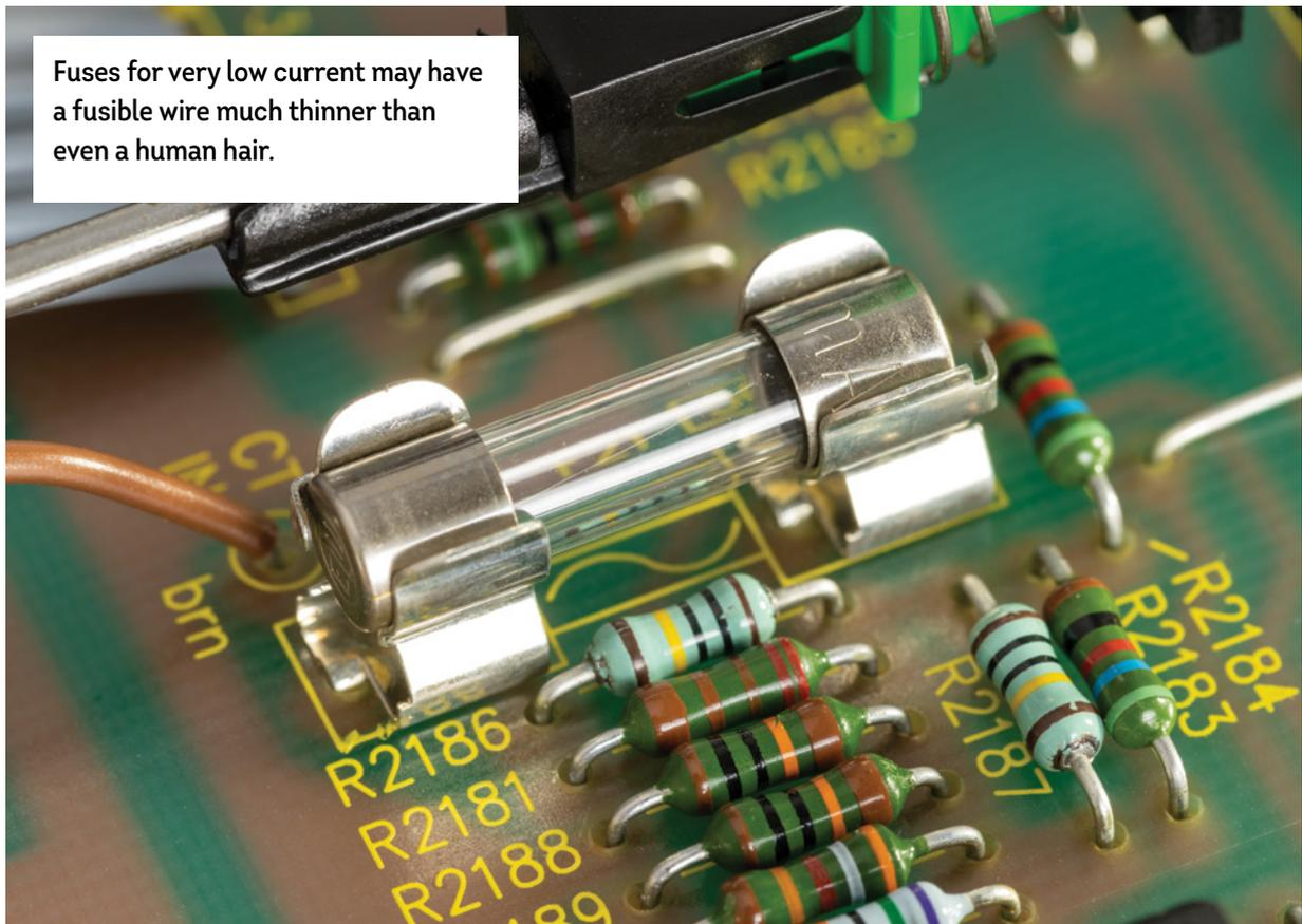
Cartridge fuses like these are found in equipment where the end user will replace the fuse. The glass case makes it easy to see when a fuse has blown.
