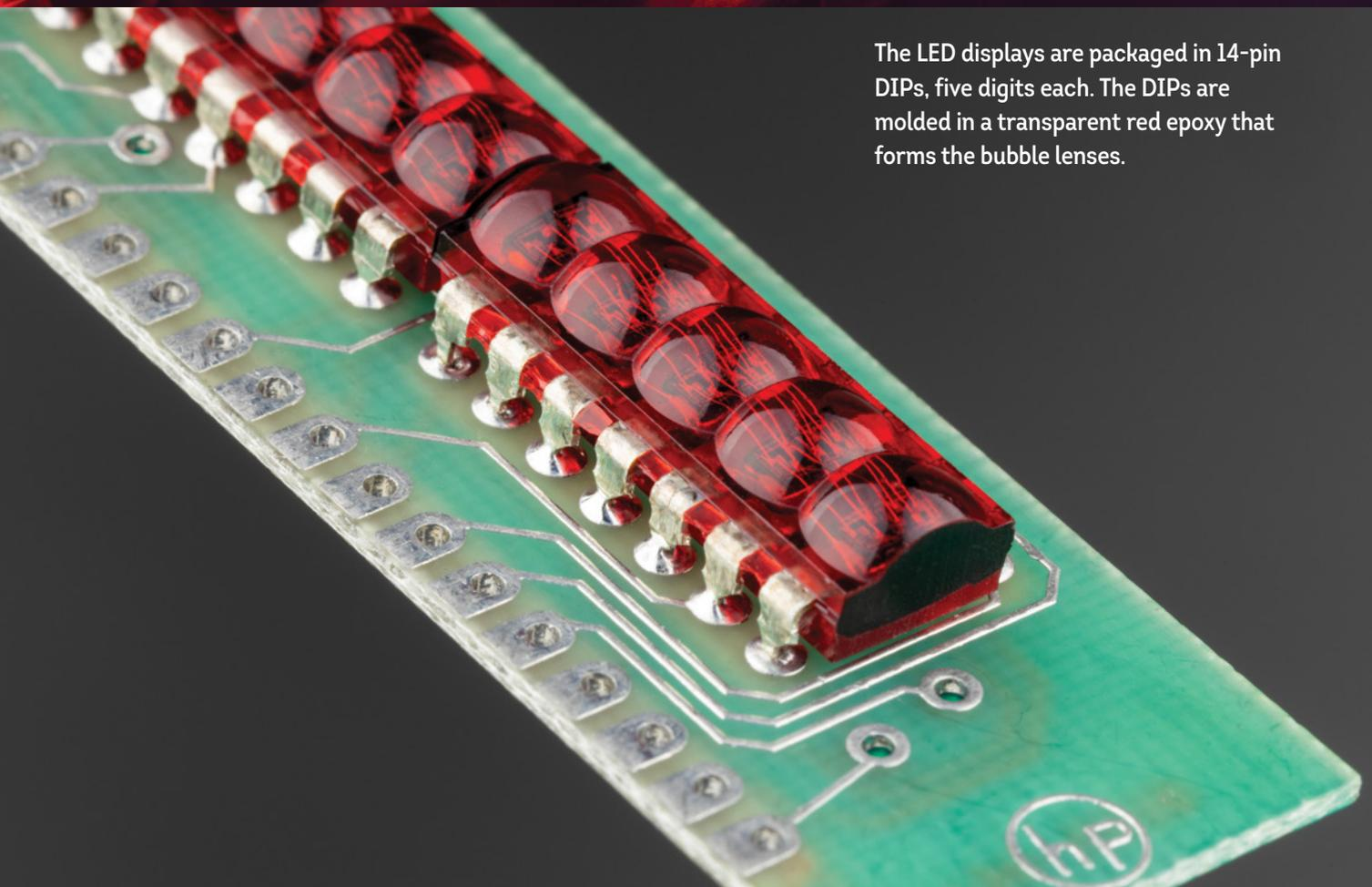
The LED displays are packaged in 14-pin DIPs, five digits each. The DIPs are molded in a transparent red epoxy that forms the bubble lenses.
