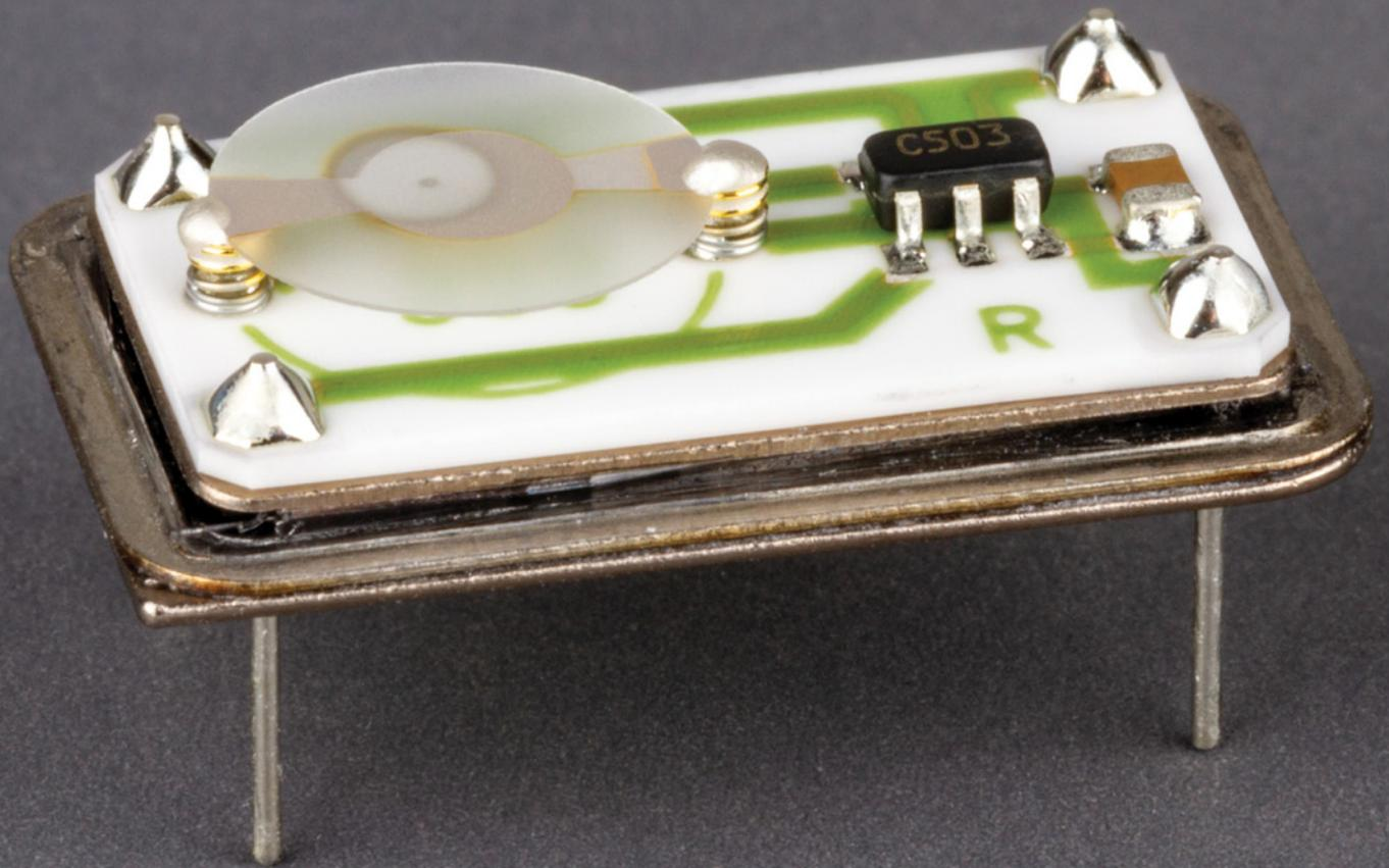
Tiny metal springs mechanically support and isolate the quartz. They also provide the electrical connection between the electrodes and the ceramic board below.
