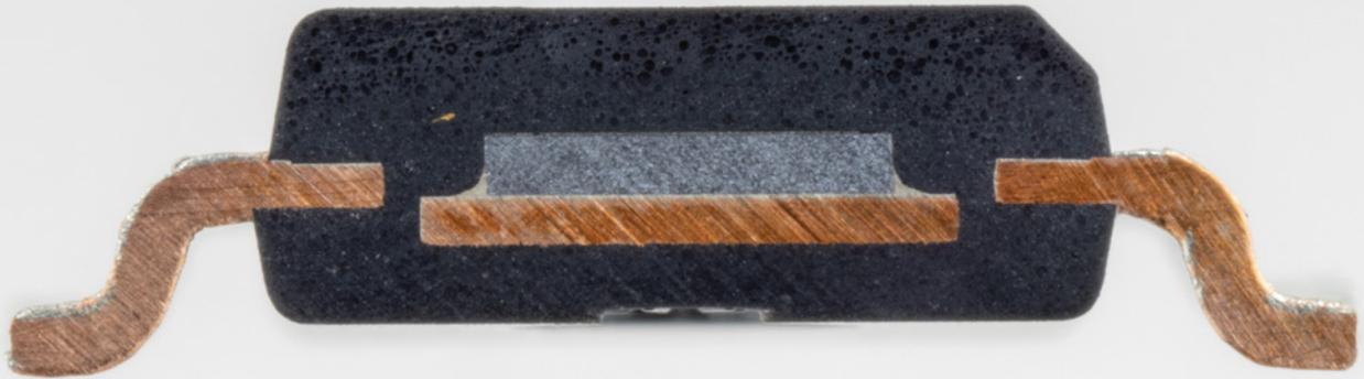
The silicon die rests on a copper lead frame in the middle of the SOIC. Tiny bond wires connect it to the various leads, but only one of them is visible in this cross section.
