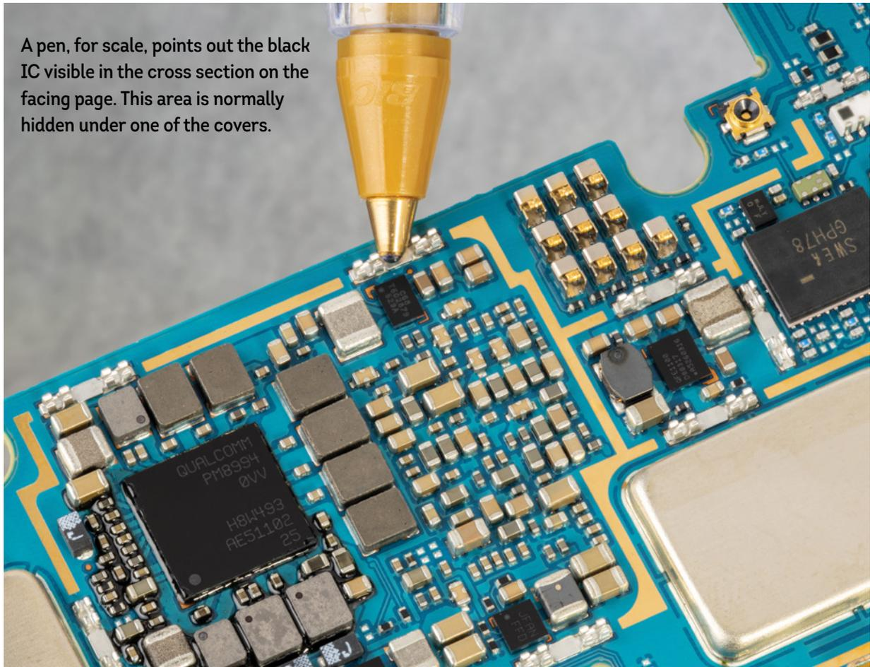
A pen, for scale, points out the black IC visible in the cross section on the facing page. This area is normally hidden under one of the covers.
