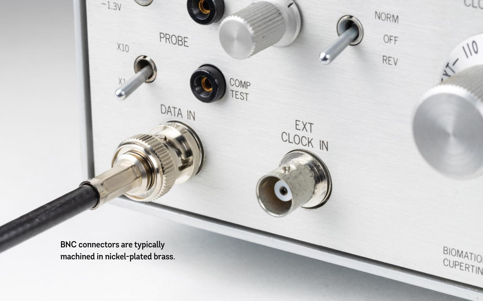
BNC connectors are typically machined in nickel-plated brass.
