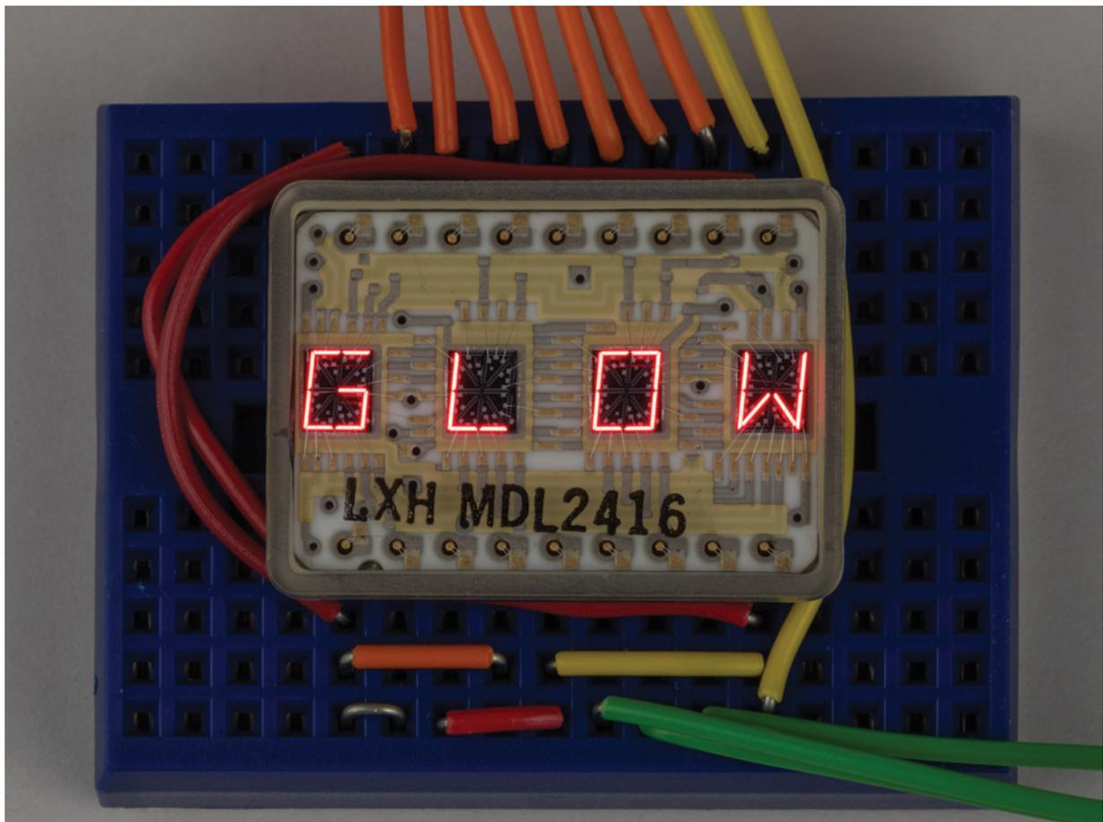
The LED chip has an extra decimal point and contact pads so it can be rotated 180 degrees and still be installed correctly.
