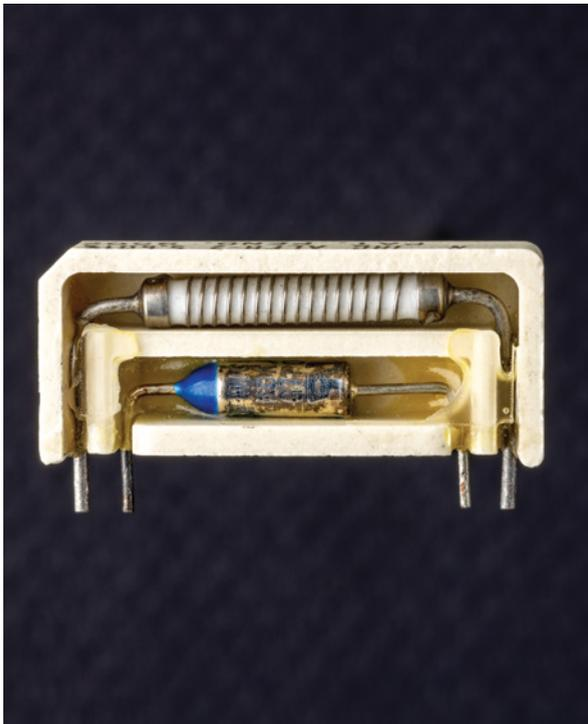
As a precaution, thermal fuses are sometimes packaged with wirewound power resistors, which are likely to be one of the hottest points in a circuit.
