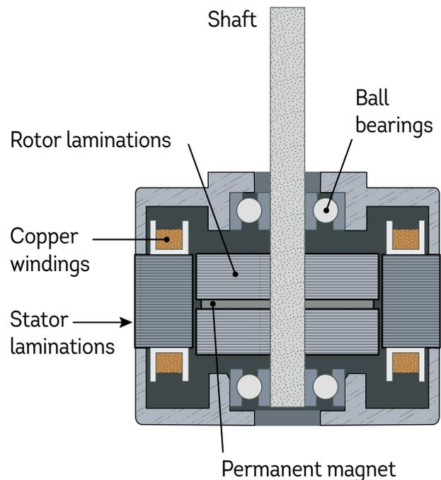
When assembled, the rotor fits neatly inside the stator, with only a thin gap between the two.
