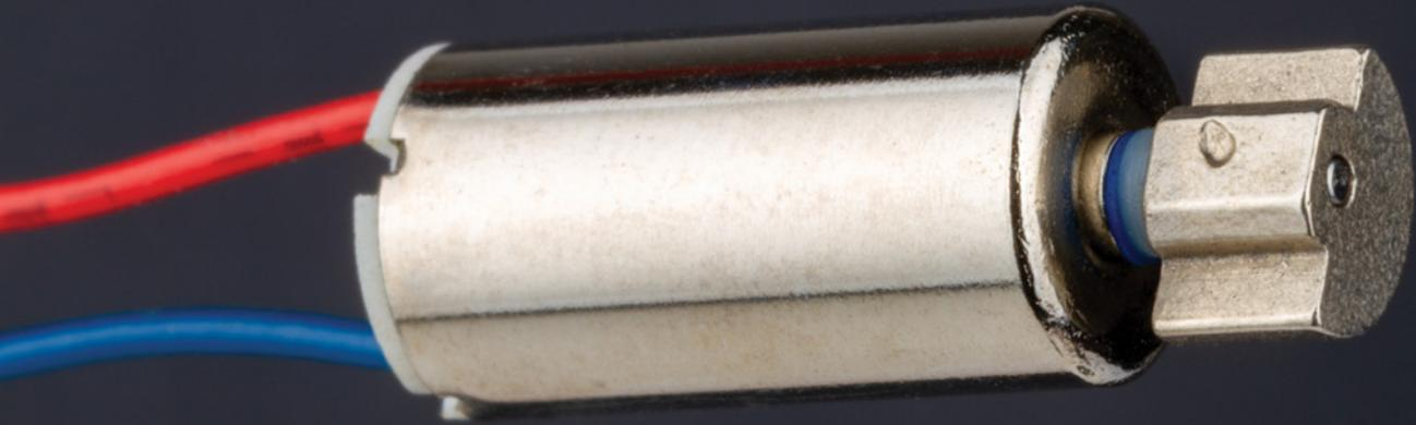
The offset weight on the output shaft of the motor causes the motor to vigorously wobble when it spins. With the motor's small size and fast rotation, we perceive only a vibration in place.
