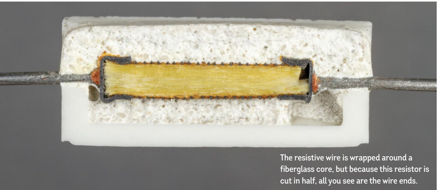
The resistive wire is wrapped around a fiberglass core, but because this resistor is cut in half, all you see are the wire ends.
