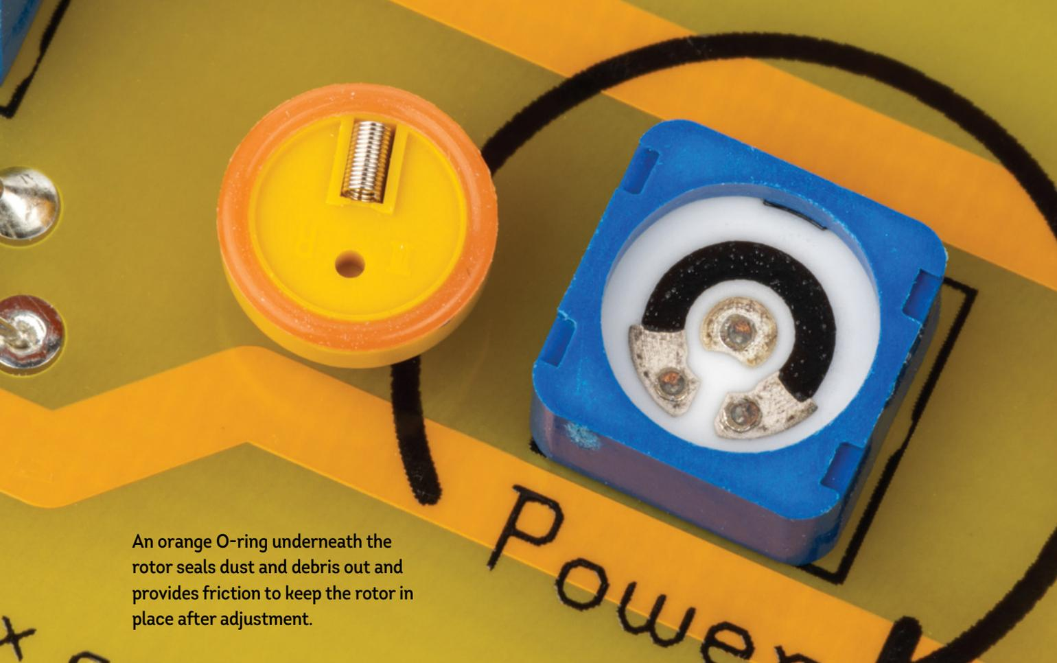
An orange O-ring underneath the rotor seals dust and debris out and provides friction to keep the rotor in place after adjustment.
