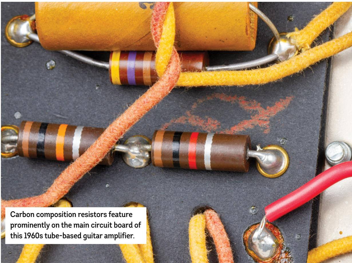
Carbon composition resistors feature prominently on the main circuit board of this 1960s tube-based guitar amplifier.
