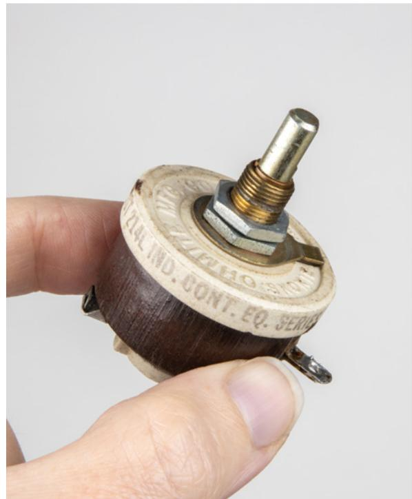
The wiper of a standard pot can be rotated about  $\frac{2}{3}$  to  $\frac{3}{4}$  of a turn, between the two fixed terminals.
