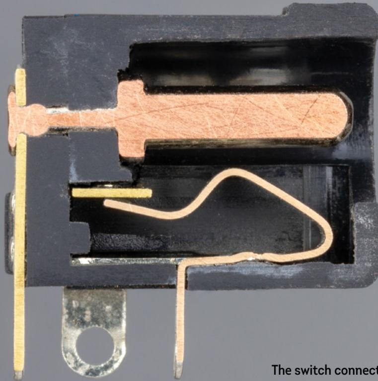
The switch connects the external terminal of the jack to a third pin, but only when the plug isn't present.
