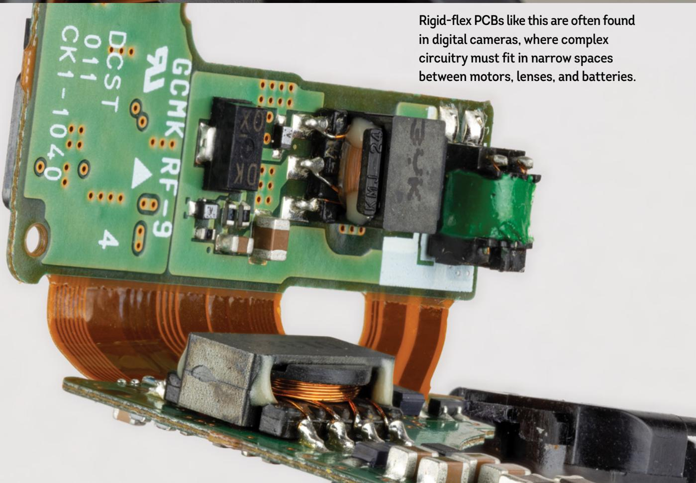
Rigid-flex PCBs like this are often found in digital cameras, where complex circuitry must fit in narrow spaces between motors, lenses, and batteries.
