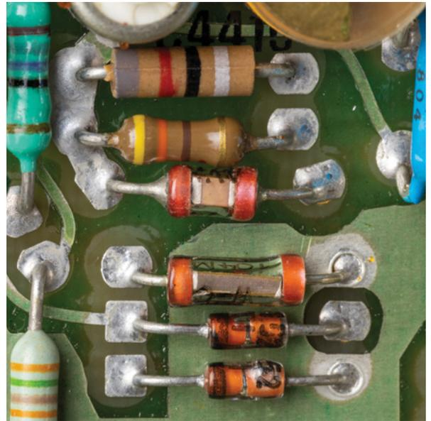
This axial-packaged MLCC, with a passing resemblance to a strawberry ice cream sandwich, has about 30 interdigitated metal layers.
