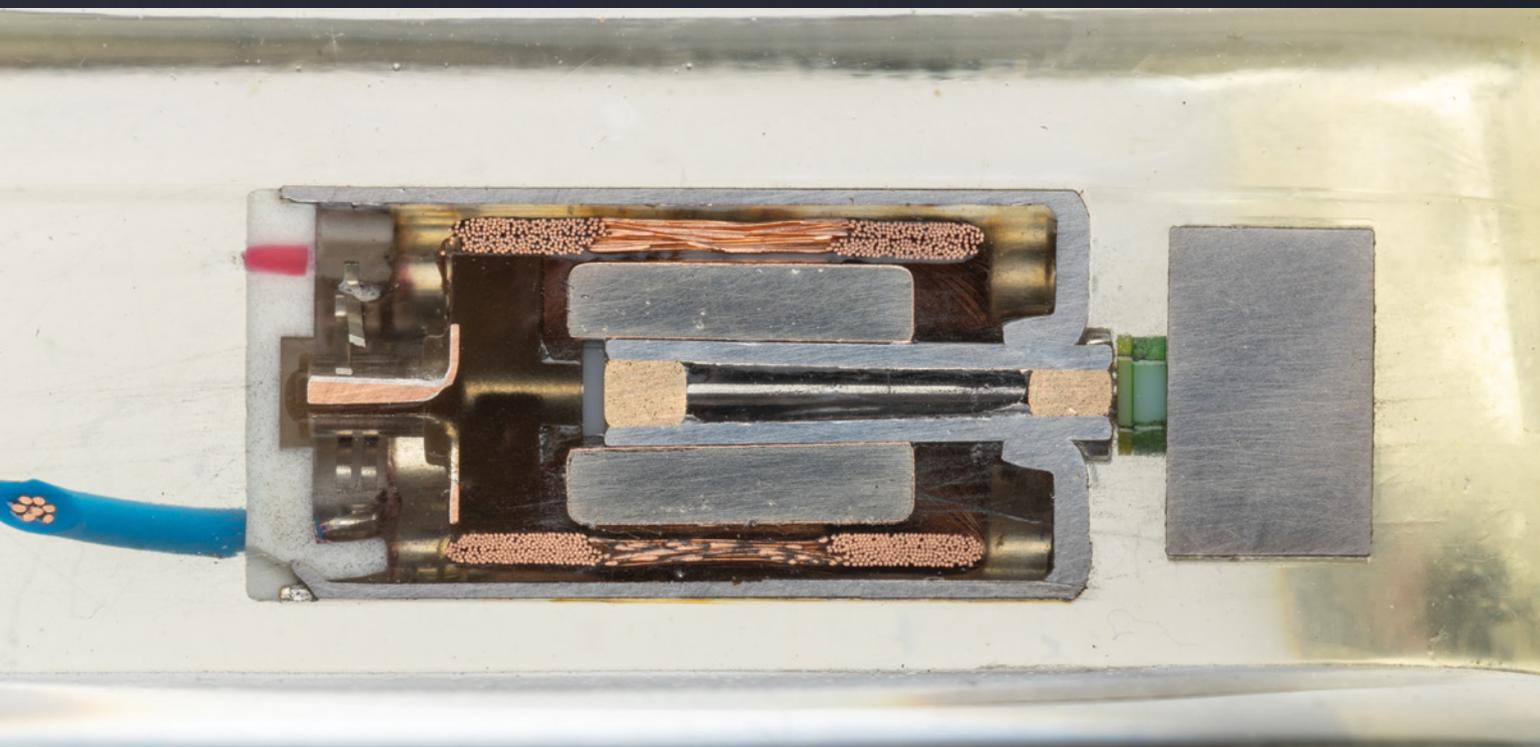
The tube-shaped inner magnet remains stationary while the copper windings rotate around it.
