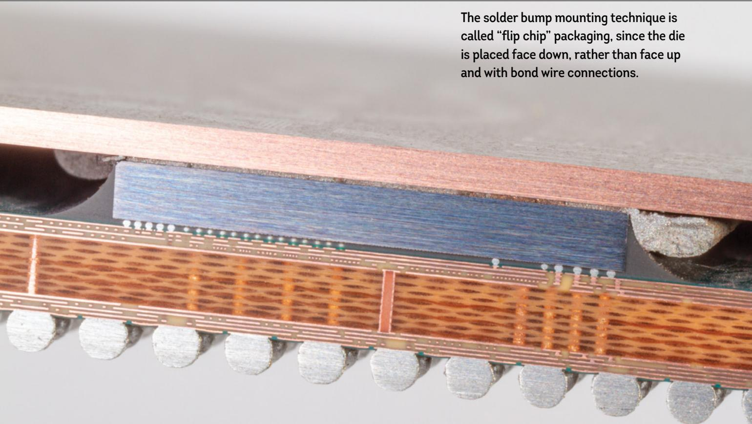
The solder bump mounting technique is called “flip chip” packaging, since the die is placed face down, rather than face up and with bond wire connections.
