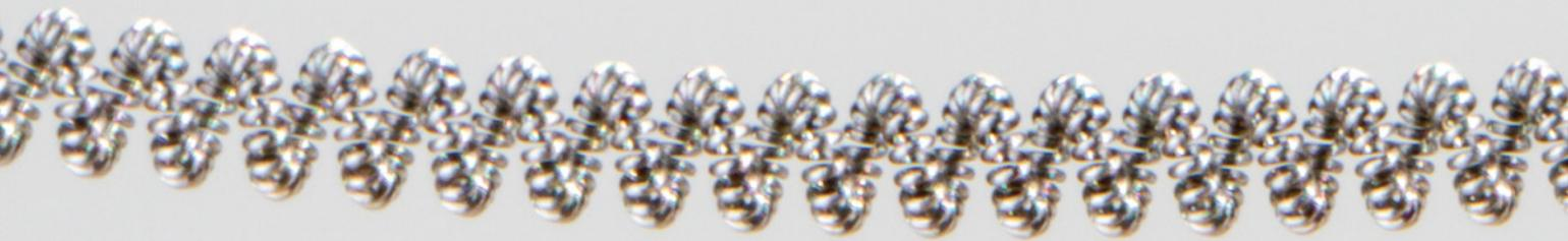
The filament is a coiled coil of remarkably fine tungsten wire.
