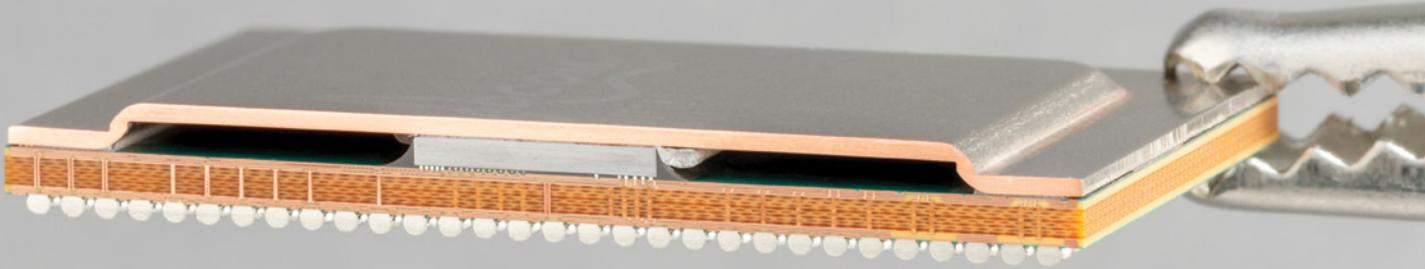
The “cap” on this SoC is a large nickel-plated copper heat spreader. It’s attached to the top of the silicon die with thermal compound.
