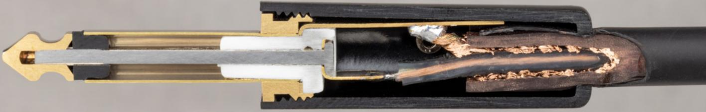
The tip of the plug is connected to the center wire of the cable while the outer sleeve is connected to the cable's outer shielding.
