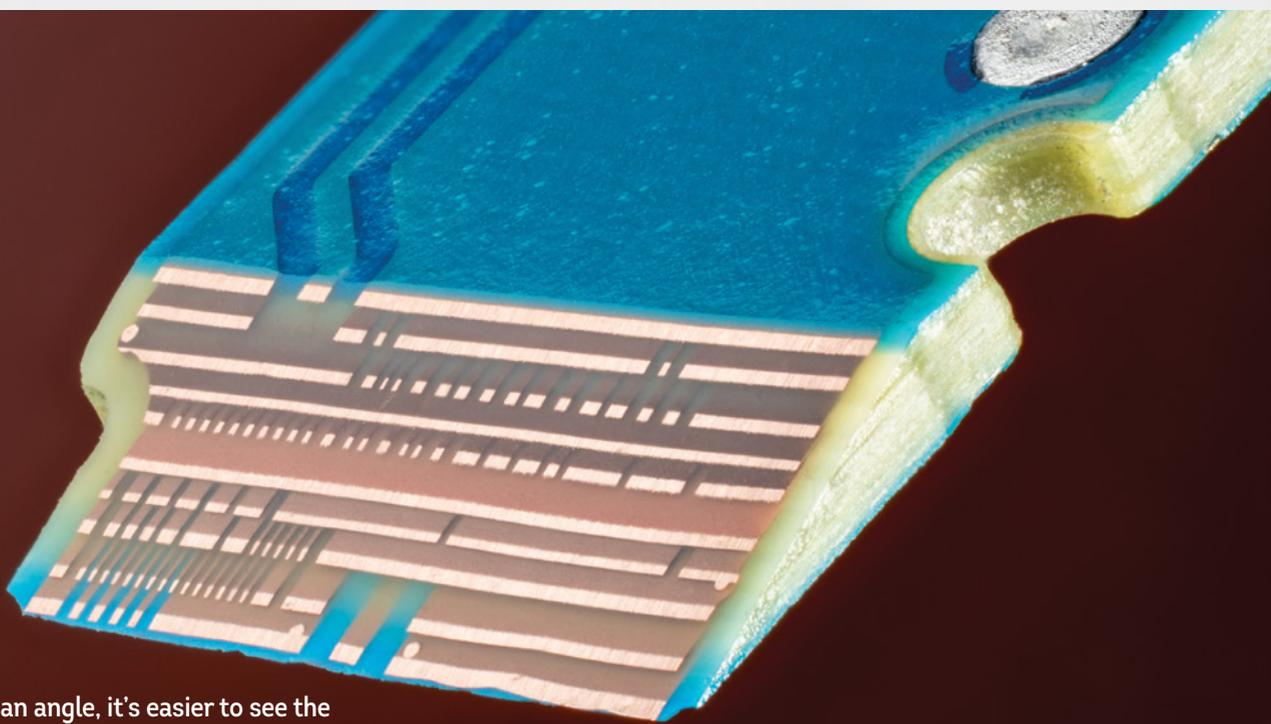
Cut at an angle, it's easier to see the three-dimensional nature of the circuit board. The circular structures are vias that have been cut through.
