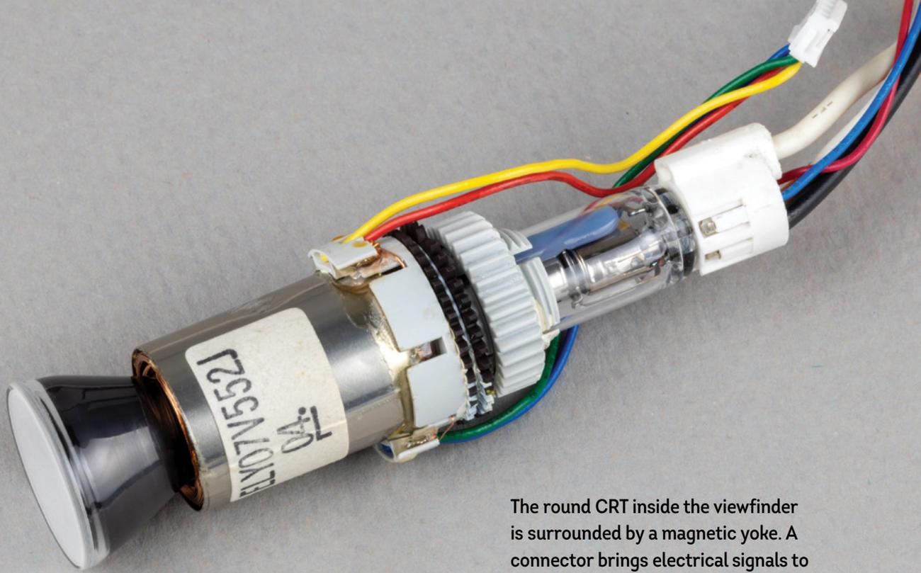
The round CRT inside the viewfinder is surrounded by a magnetic yoke. A connector brings electrical signals to the pins of the tube.
