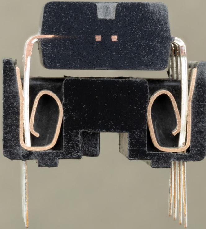
Dual-wipe sockets have springy contacts that grip each pin of the integrated circuit package.
