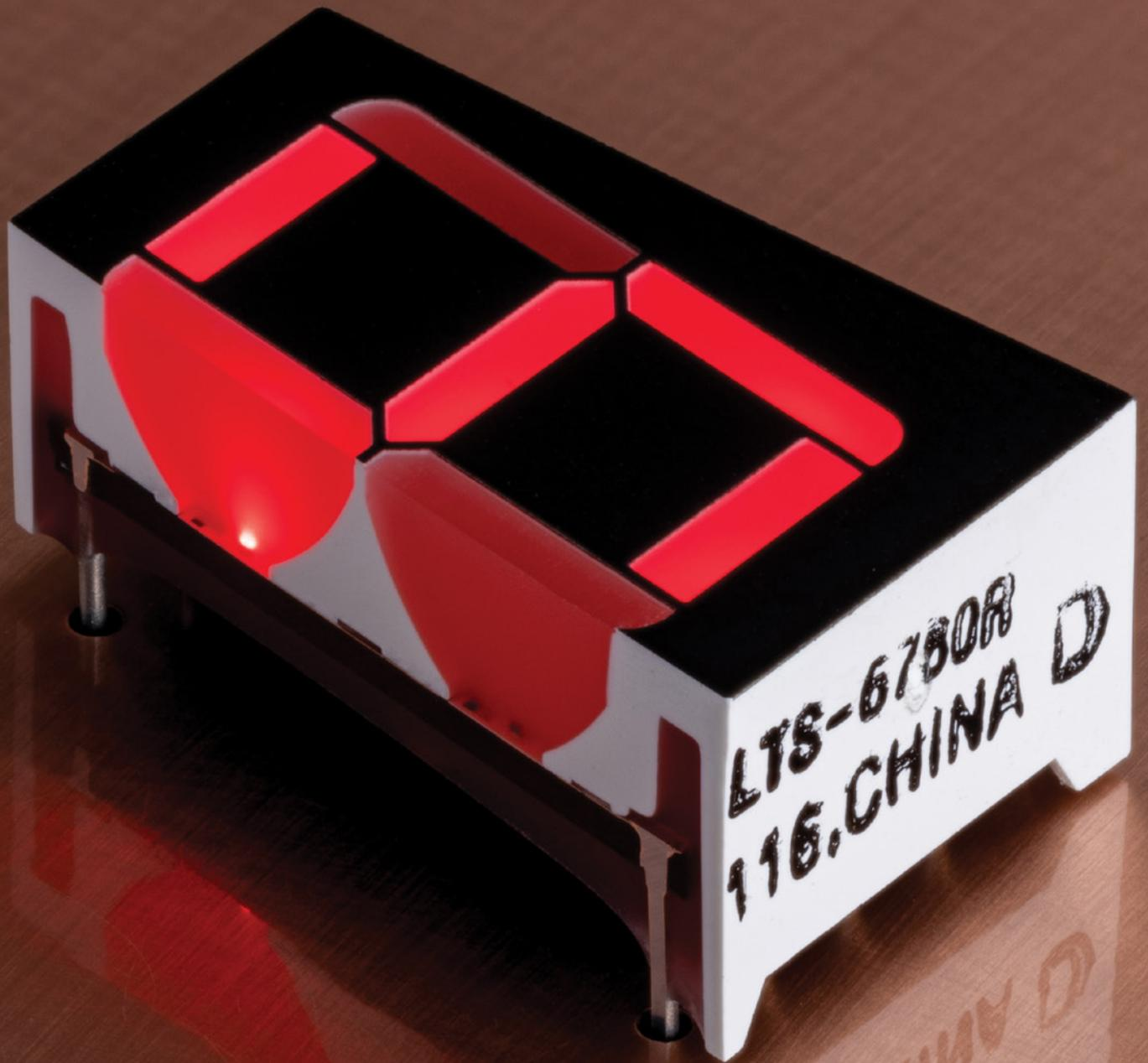
The slightly cloudy red epoxy that forms the lenses diffuses the light from the LEDs so that each lit segment appears evenly illuminated.
