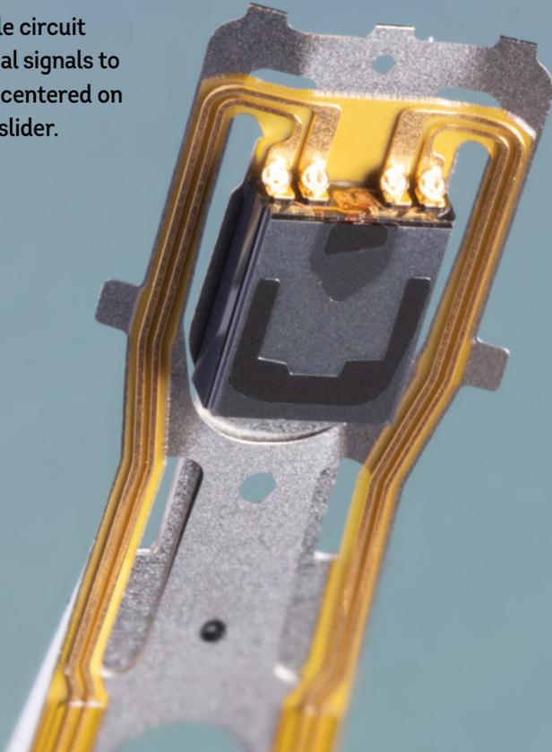
The red thin-film write head coil is at the center bottom of the slider face. The two copper rectangles behind it are part of the GMR sensor read head.
