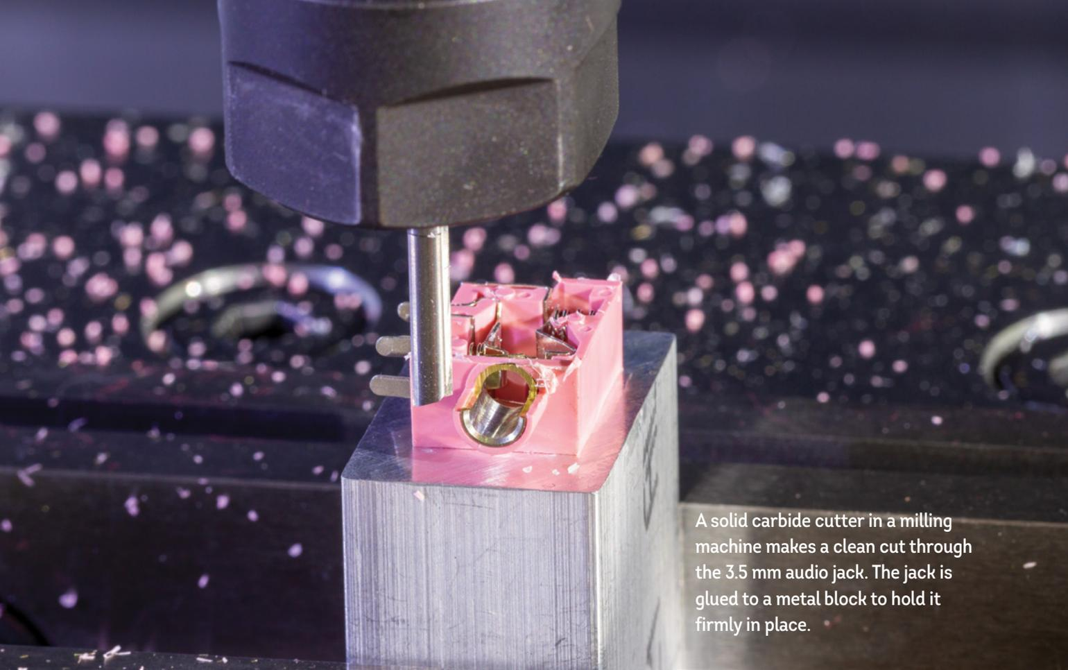
A solid carbide cutter in a milling machine makes a clean cut through the 3.5 mm audio jack. The jack is glued to a metal block to hold it firmly in place.
