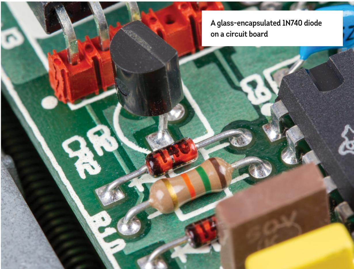
A glass-encapsulated 1N740 diode on a circuit board
