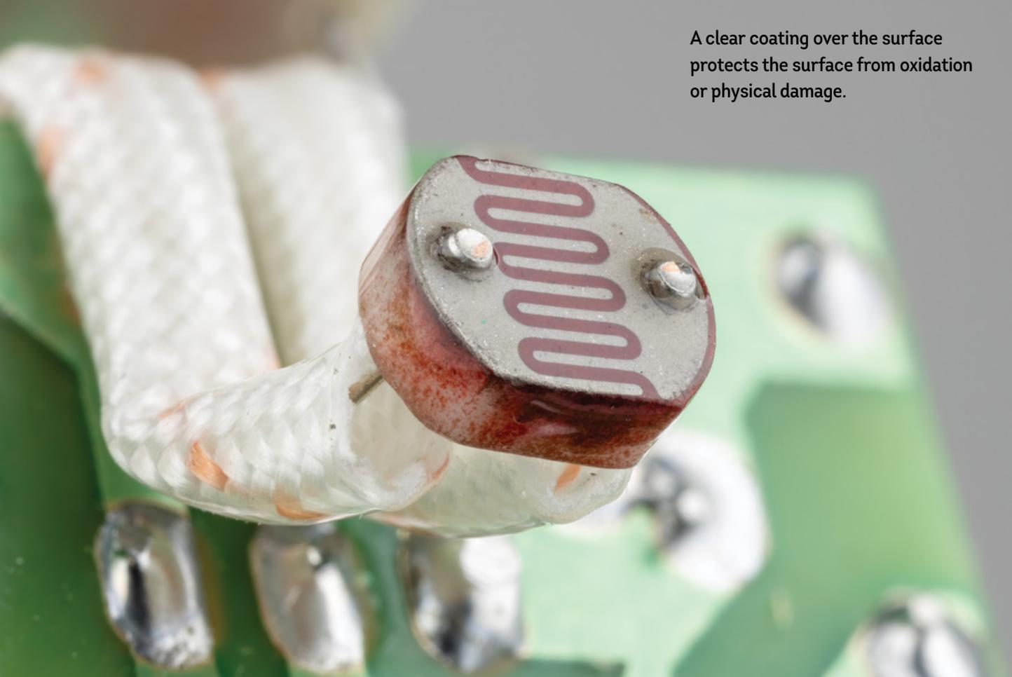
A clear coating over the surface protects the surface from oxidation or physical damage.
