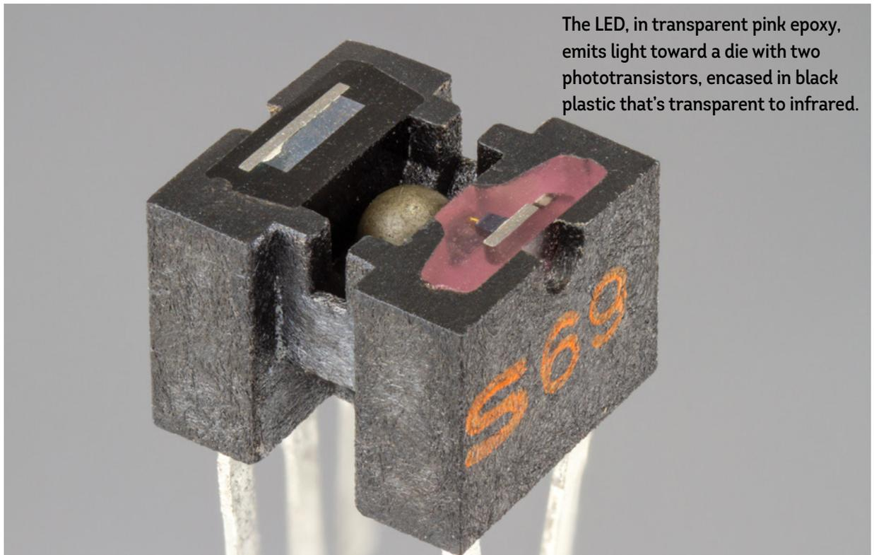
The LED, in transparent pink epoxy, emits light toward a die with two phototransistors, encased in black plastic that's transparent to infrared.
