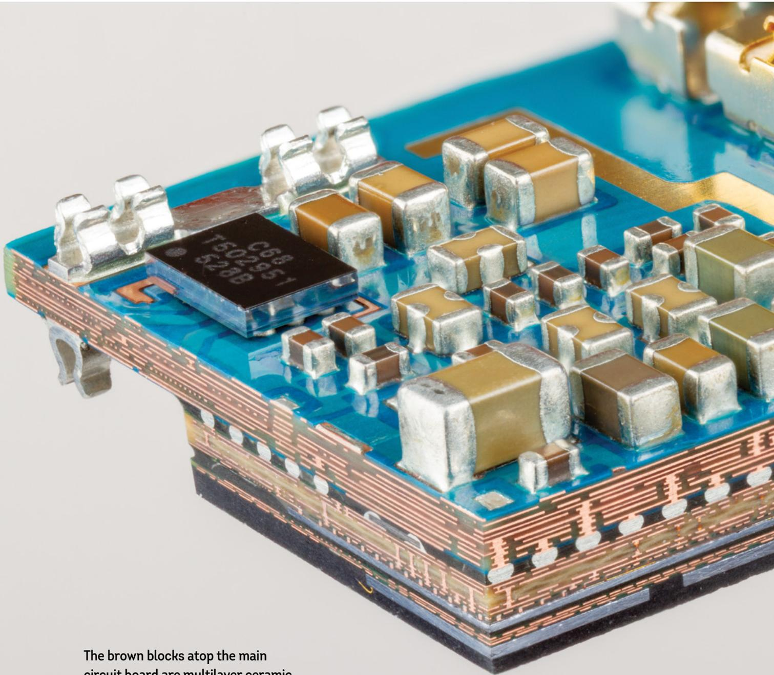
The brown blocks atop the main circuit board are multilayer ceramic capacitors (MLCCs).
