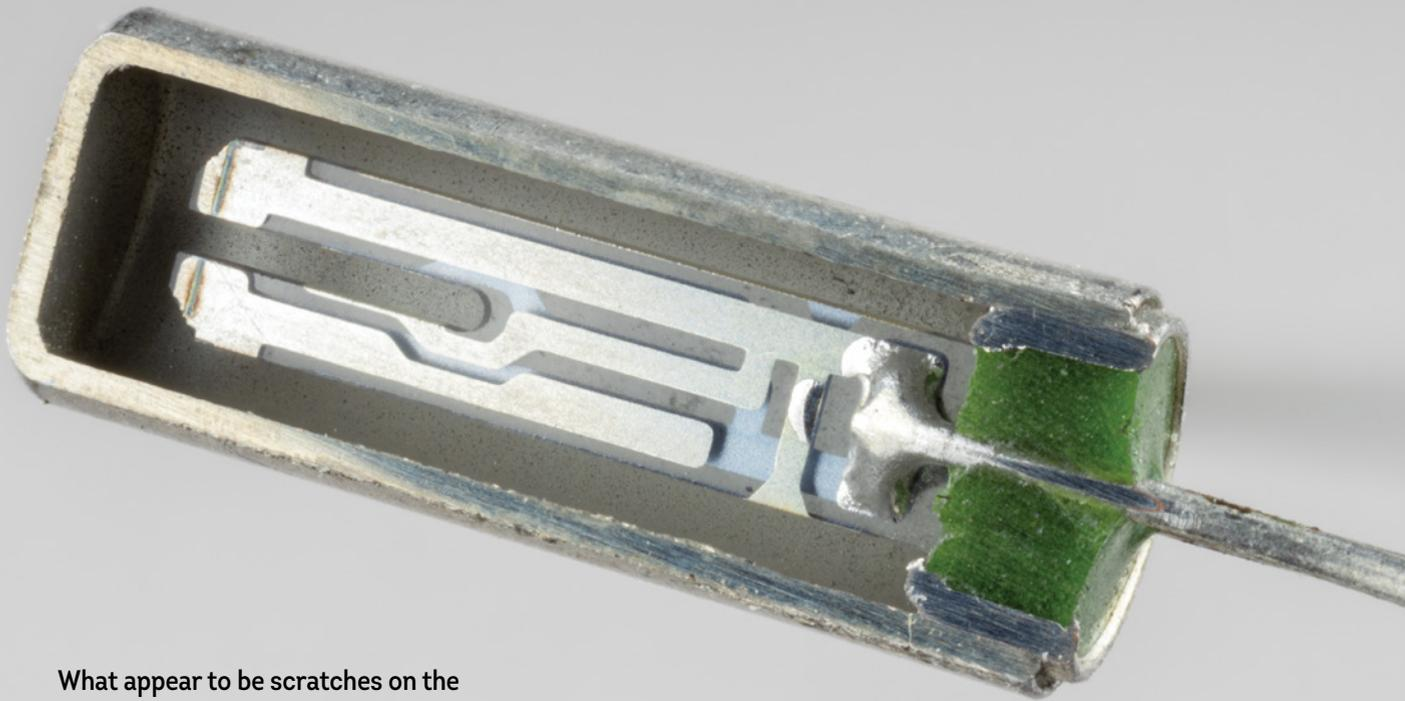
What appear to be scratches on the tips of the tuning fork are actually laser trim marks from a process that fine-tunes the frequency.
