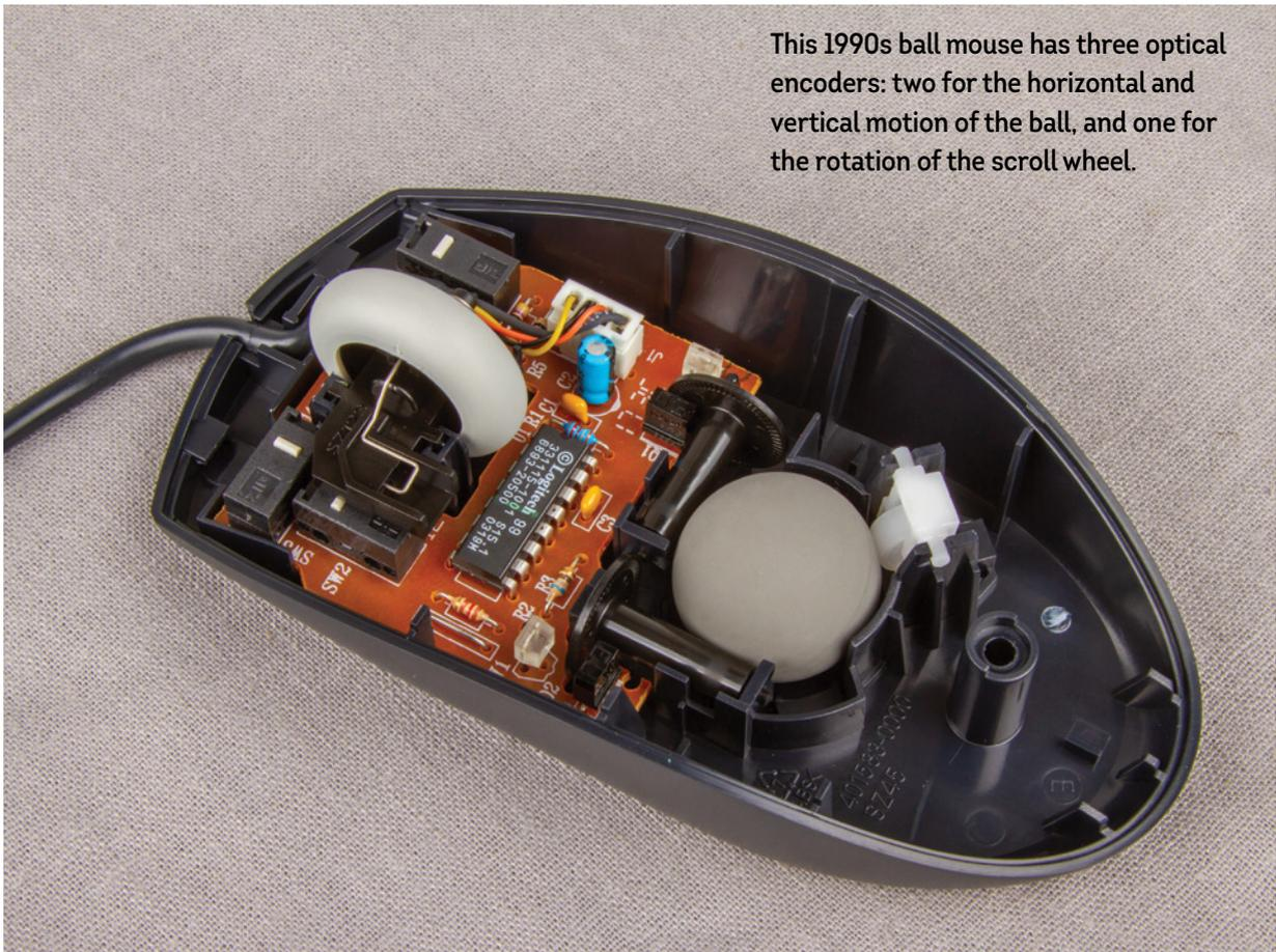
This 1990s ball mouse has three optical encoders: two for the horizontal and vertical motion of the ball, and one for the rotation of the scroll wheel.
