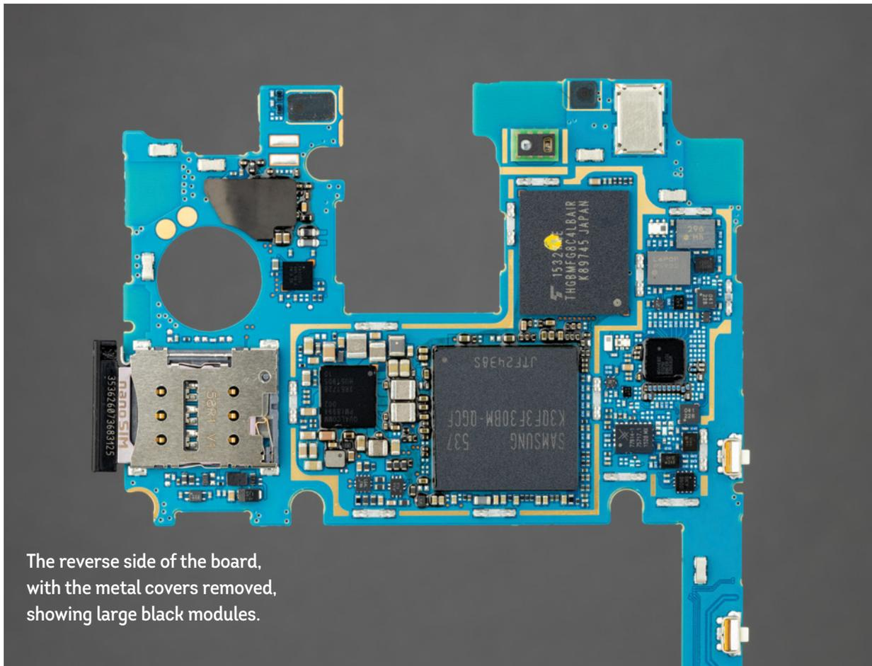
The reverse side of the board, with the metal covers removed, showing large black modules.
