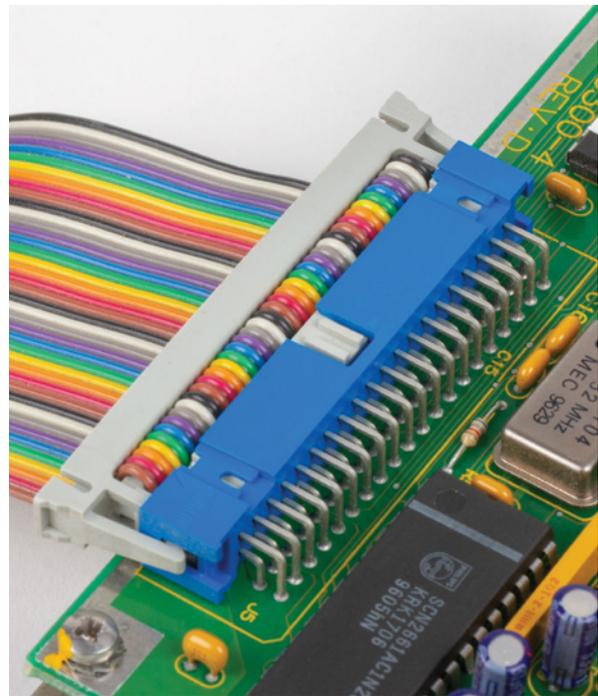
Every other wire is pierced in one row of the IDC plug. With two rows of blades, every wire connects to a mating pin.
