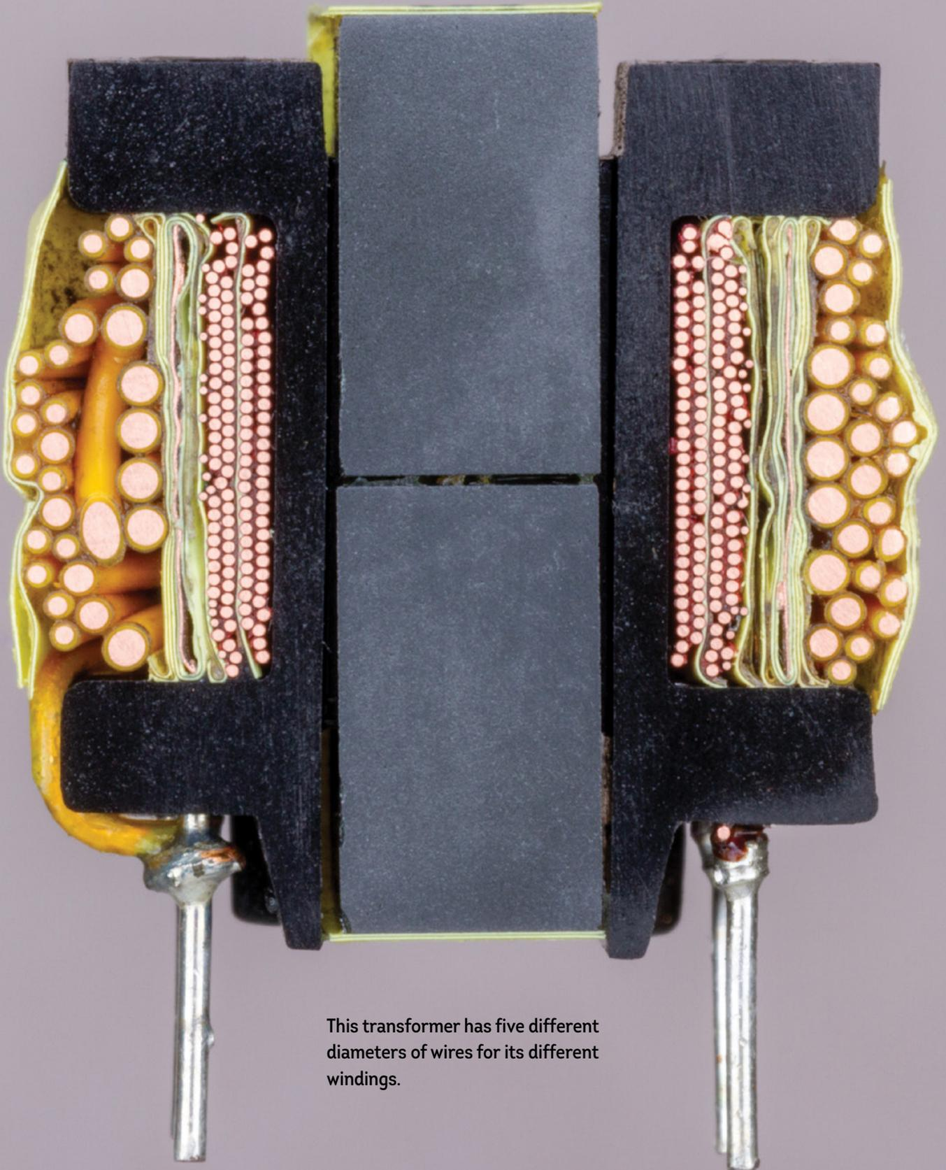
This transformer has five different diameters of wires for its different windings.
