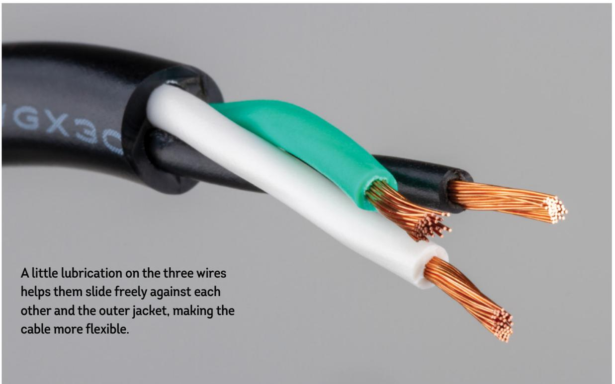
A little lubrication on the three wires helps them slide freely against each other and the outer jacket, making the cable more flexible.
