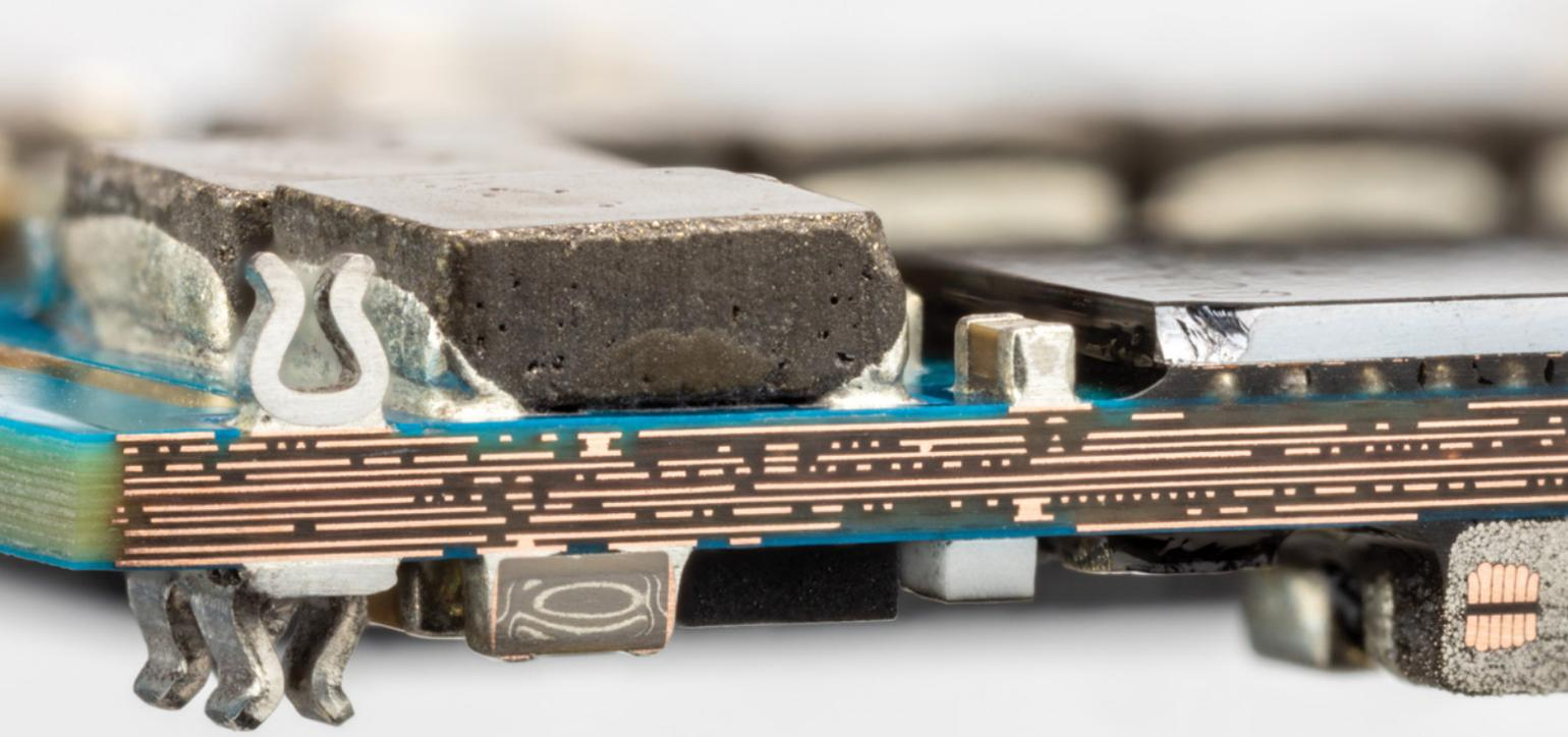
This ten-layer smartphone PCB has blind and buried vias making connections between the different layers, visible as vertical copper pillars connecting the layers.
