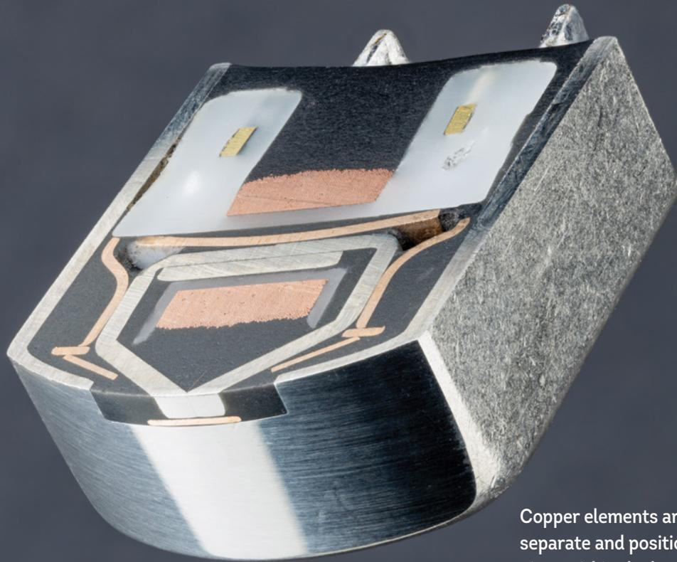
Copper elements are used to separate and position the iron pole piece within the head, isolating the magnetic circuit components.
