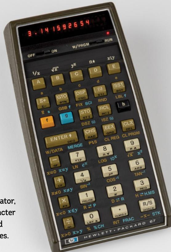
This Hewlett-Packard 67 calculator, released in 1976, has a 15-character LED “bubble” display, so called because of the bubble-like lenses.
