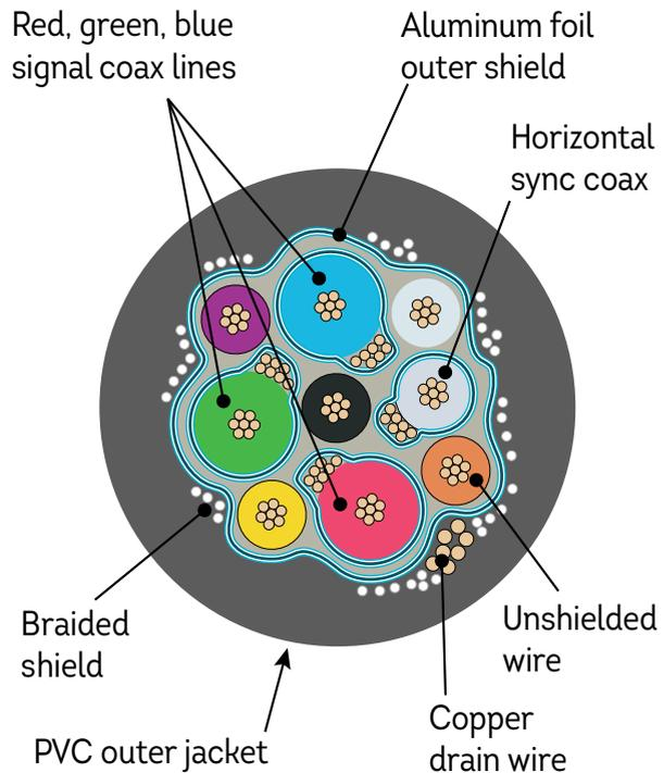
The outer shield of this cable is aluminum, with a stranded copper drain wire added.
