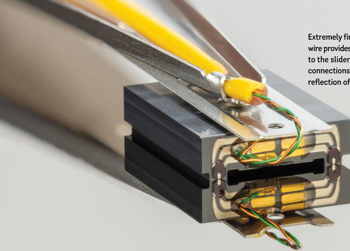
Extremely fine lacquered magnet wire provides electrical connections to the slider. The soldered connections are visible in the reflection off the drive platter.
