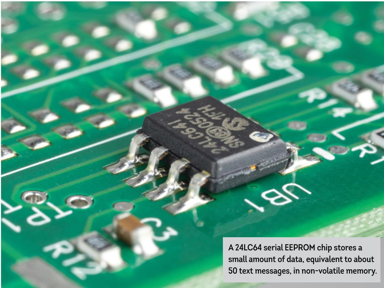
A 24LC64 serial EEPROM chip stores a small amount of data, equivalent to about 50 text messages, in non-volatile memory.
