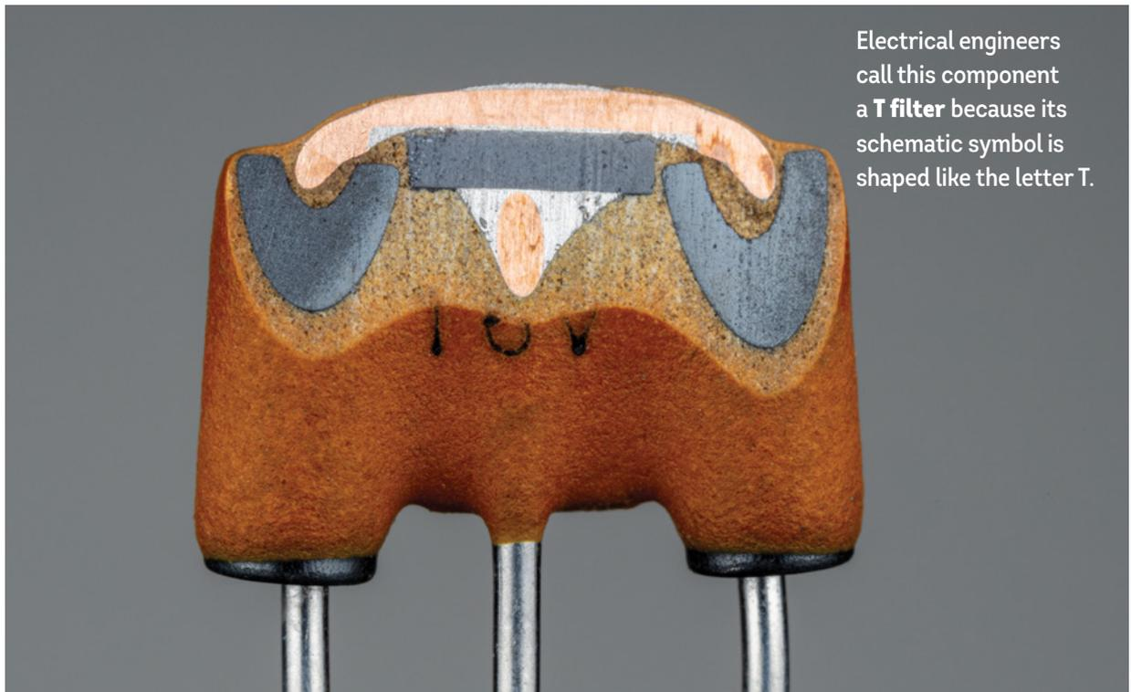
Electrical engineers call this component a **T filter** because its schematic symbol is shaped like the letter T.
