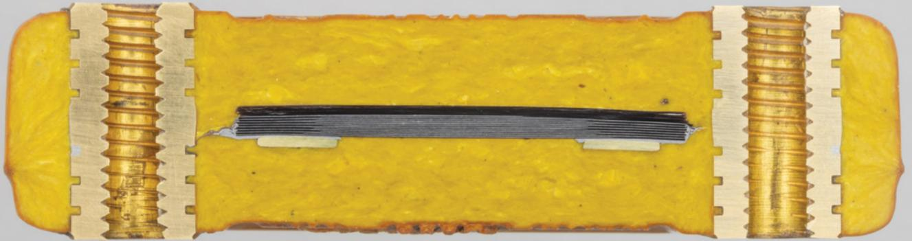
With a foreshortened perspective, we can see the interdigitated layers of this capacitor: shiny silver layers separated by darker mica layers.
