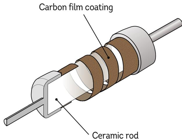
The carbon film is relatively thin. In cross section, the grooves are visible only as indentations in the ceramic rod.
