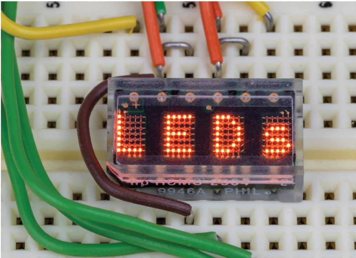
The LED dies are arranged in a matrix, with circuit board traces defining the columns in this view and daisy-chained bond wires defining the rows.
