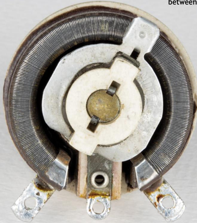
Most of the wrapped wire is covered with vitreous enamel, similar to a pottery glaze. Only the surface that contacts the wiper has exposed wire.
