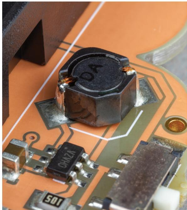
Small ferrite-core inductors are commonly used as a “flywheel” for current in DC-DC voltage converters.
