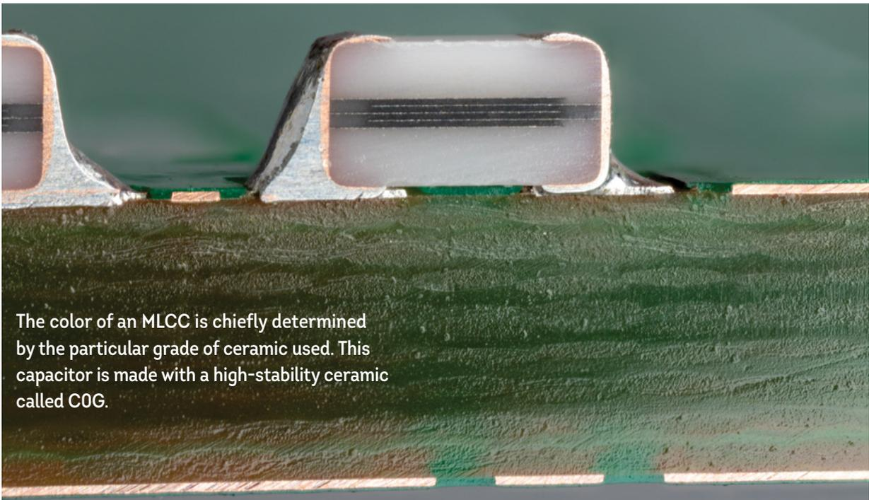
The color of an MLCC is chiefly determined by the particular grade of ceramic used. This capacitor is made with a high-stability ceramic called COG.
