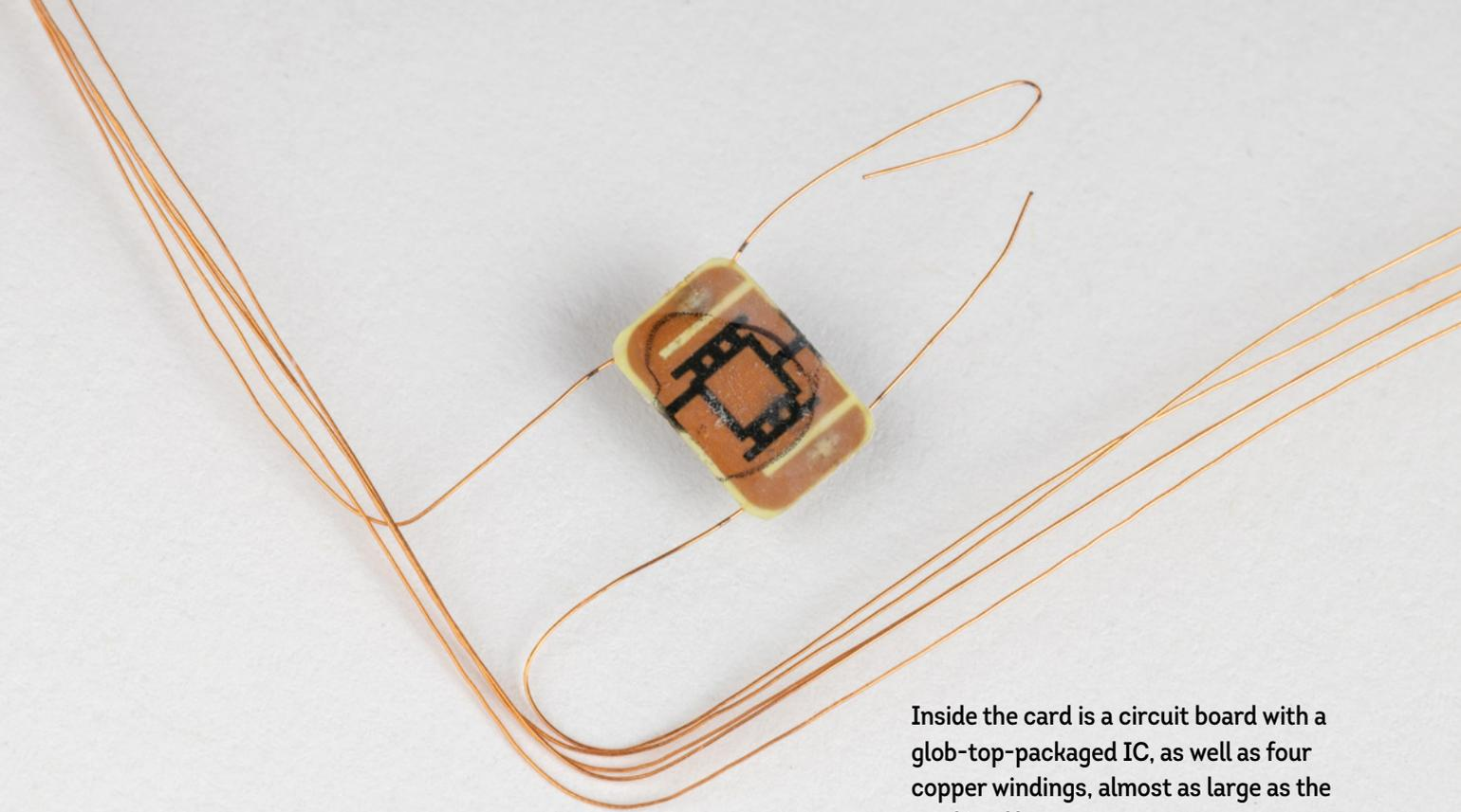
Inside the card is a circuit board with a glob-top-packaged IC, as well as four copper windings, almost as large as the card itself.
