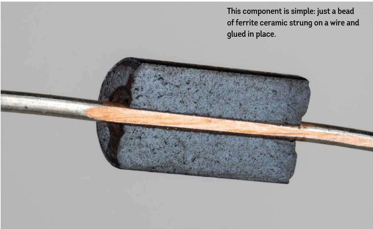
This component is simple: just a bead of ferrite ceramic strung on a wire and glued in place.
