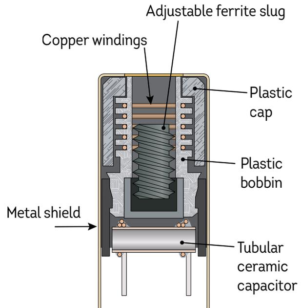
The cut silvery tube at the bottom of the IF transformer is an old-style tubular ceramic capacitor, a type common in the 1960s.
