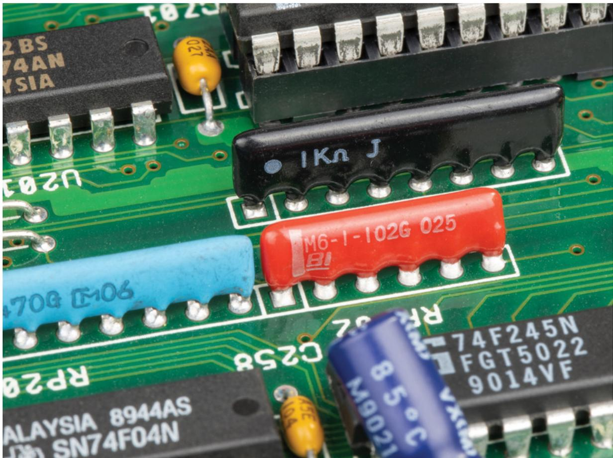
This is a *single in-line resistor array*, or *SIL*, where all the terminals are arranged in a straight line. It has four independent resistors that aren't connected to each other.
