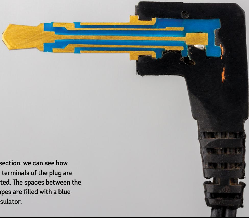
In cross section, we can see how the three terminals of the plug are constructed. The spaces between the brass shapes are filled with a blue plastic insulator.
