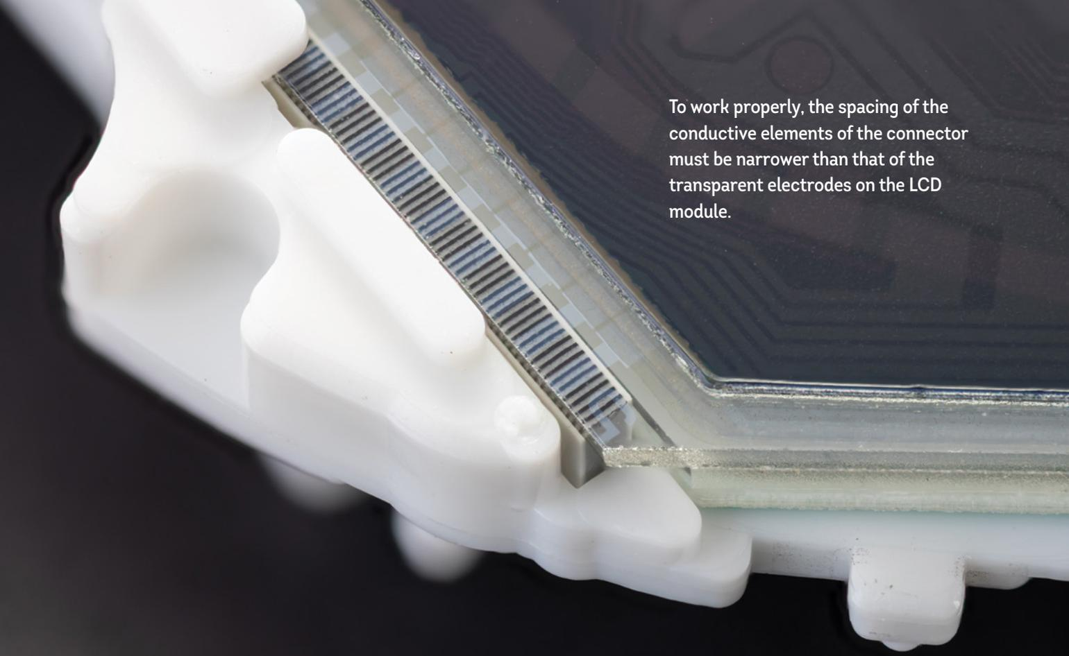
To work properly, the spacing of the conductive elements of the connector must be narrower than that of the transparent electrodes on the LCD module.
