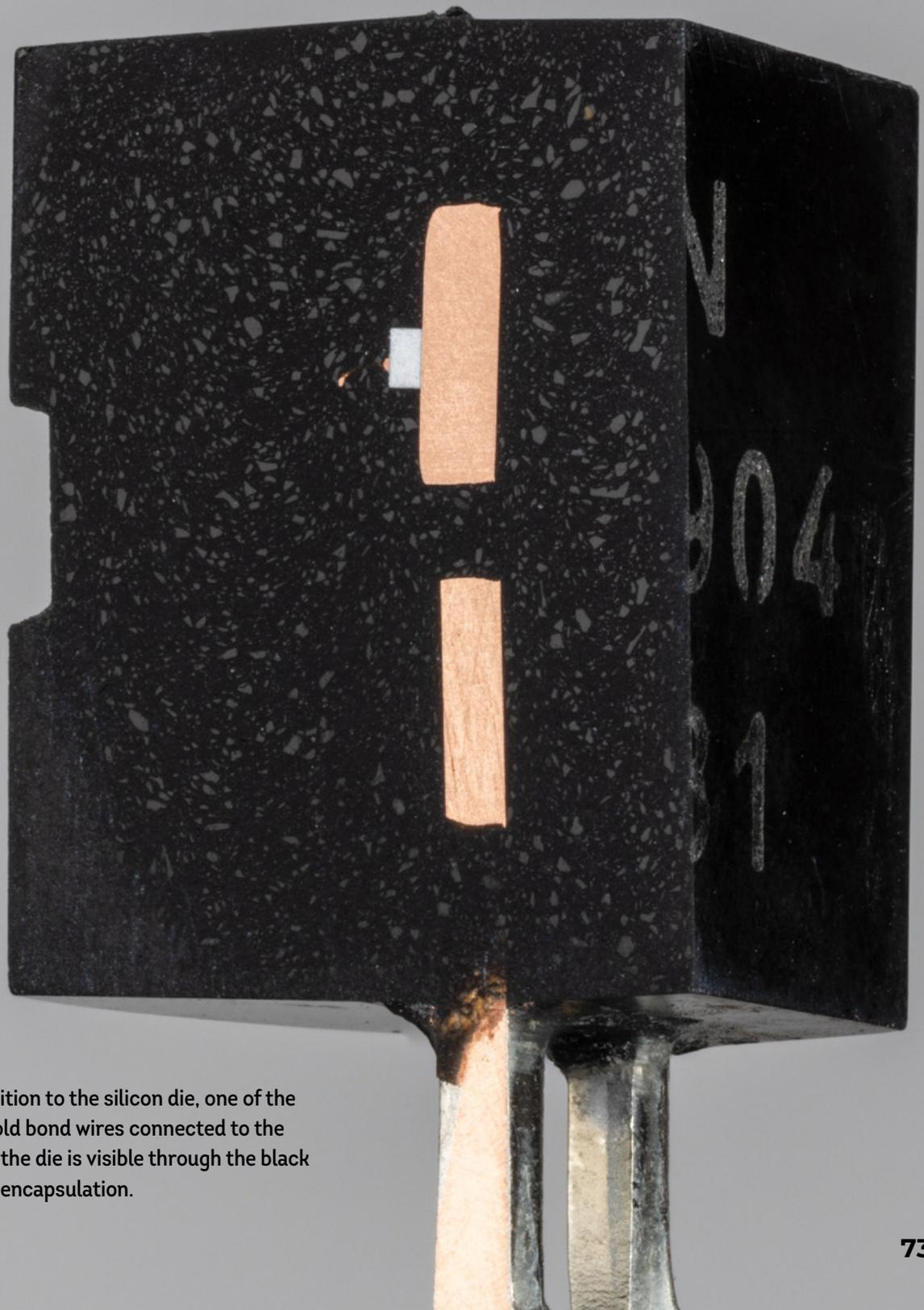
In addition to the silicon die, one of the two gold bond wires connected to the top of the die is visible through the black epoxy encapsulation.
