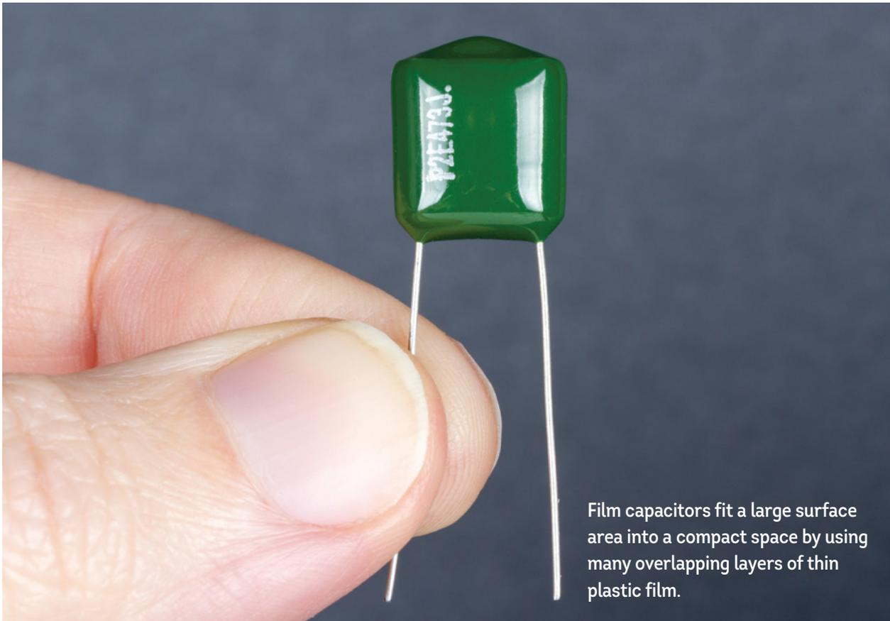
Film capacitors fit a large surface area into a compact space by using many overlapping layers of thin plastic film.
