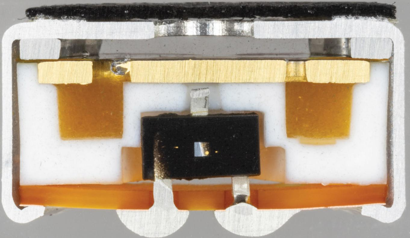
This cross section was made by embedding the microphone in clear resin before cutting it. The cut goes through the die and bond wires of the transistor in the black package.
