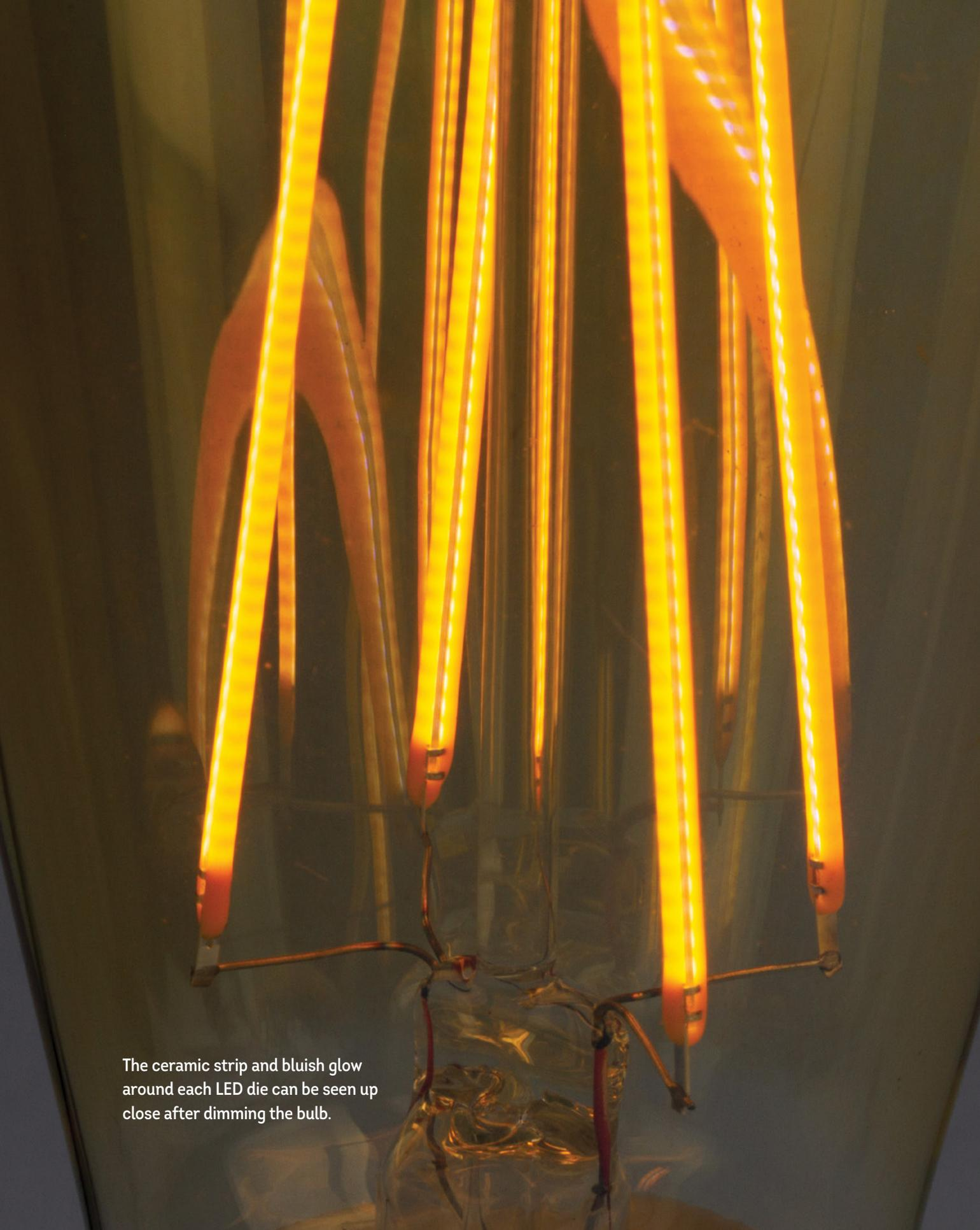
The ceramic strip and bluish glow around each LED die can be seen up close after dimming the bulb.
