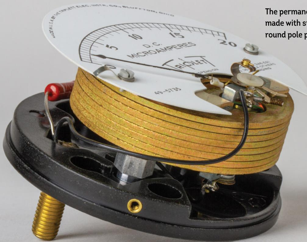
The permanent magnet is made with stacks of thick, round pole pieces.
