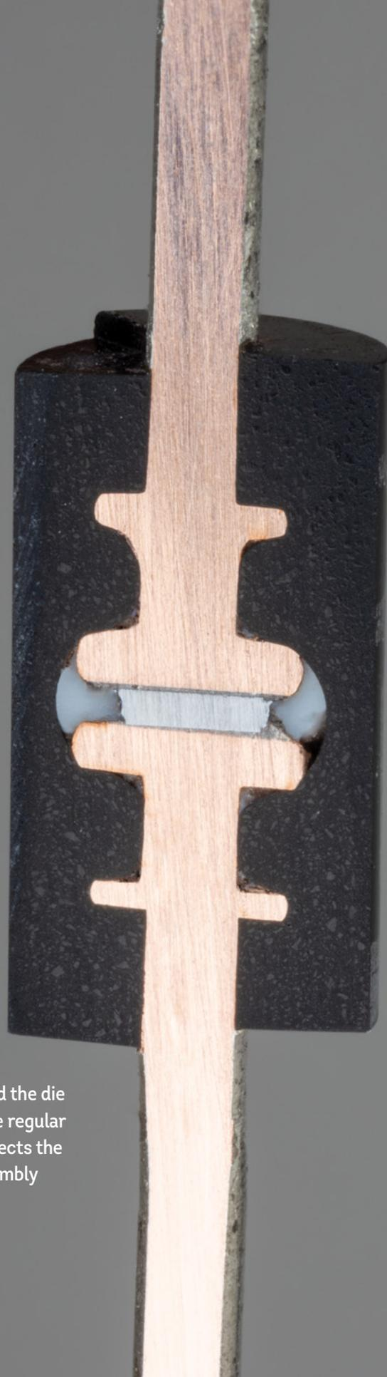
The white substance around the die is silicone rubber, much like regular household caulking. It protects the silicon chip during the assembly process.
