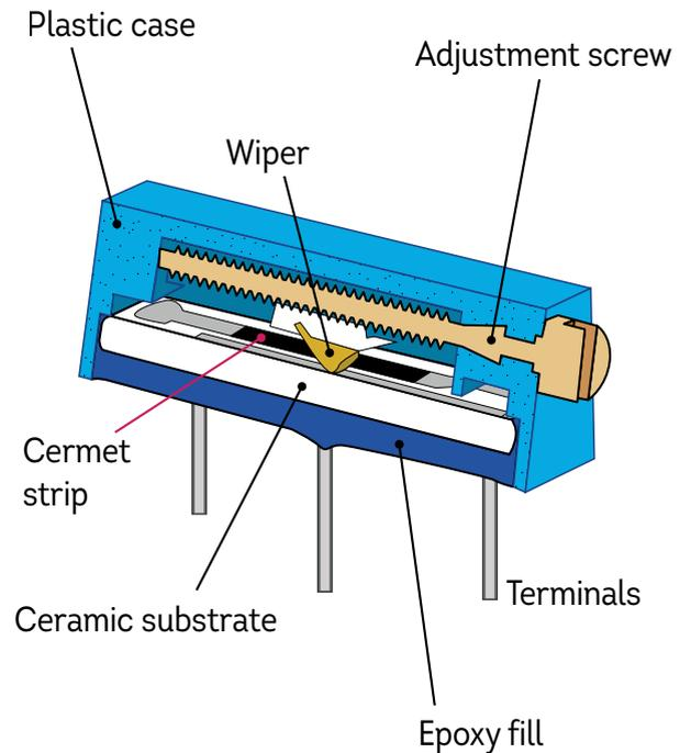
While it isn't obvious from the outside of the device, the adjustment screw is electrically insulated from all three pins of the component.
