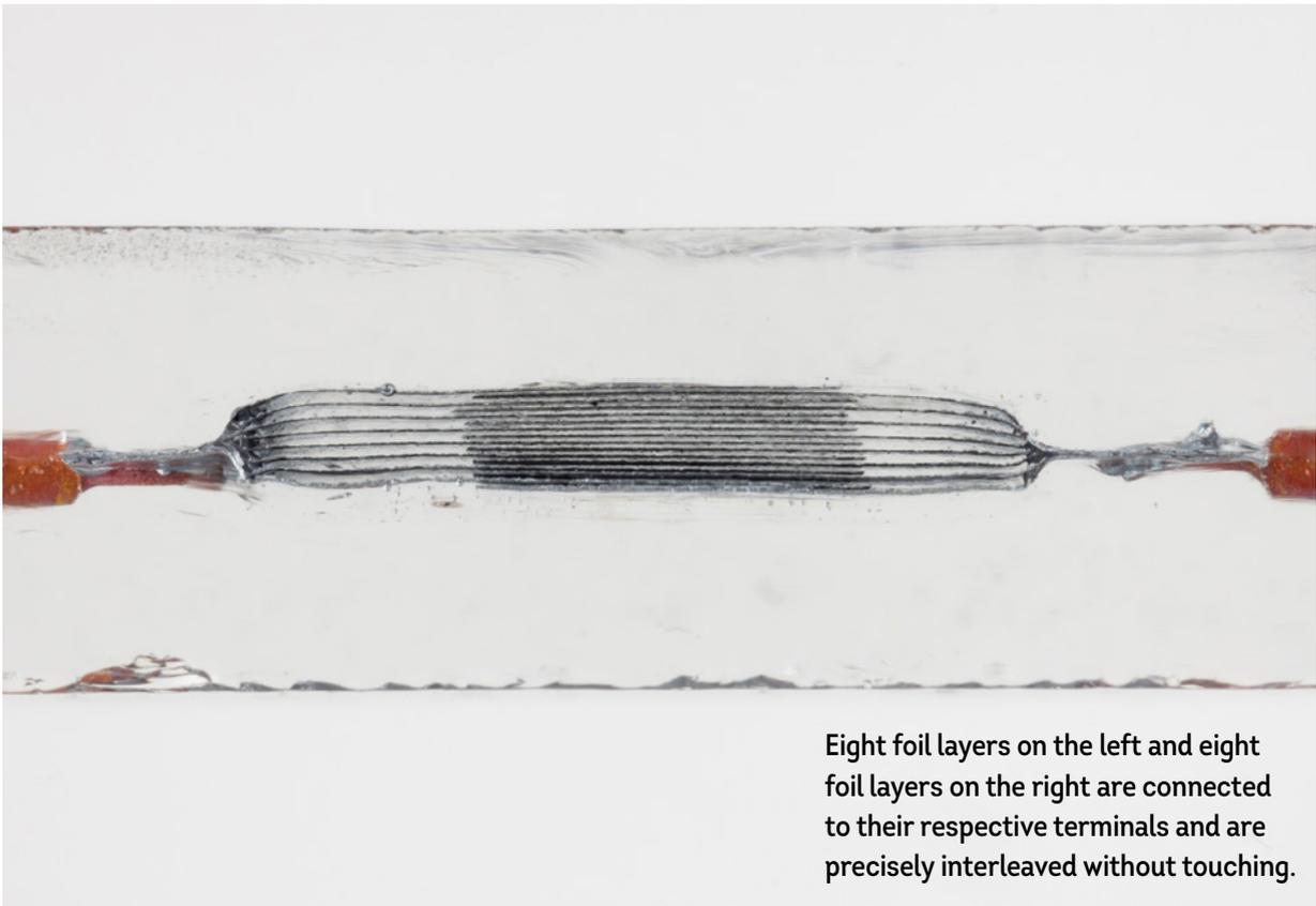
Eight foil layers on the left and eight foil layers on the right are connected to their respective terminals and are precisely interleaved without touching.
