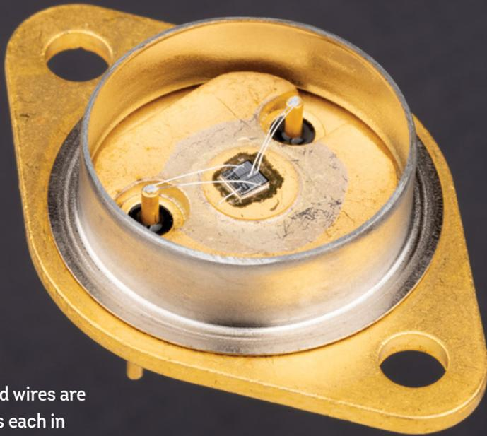
The input and output bond wires are configured with two wires each in parallel, which doubles their current-carrying capacity.
