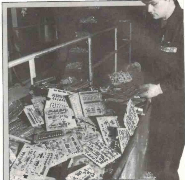
The start of the process: Piles of unwanted circuit boards are sorted before being fed into the crusher.
