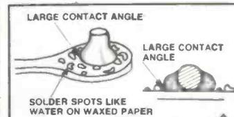
Figure 15. Dewetting. The solder appears to flow properly, then withdraws when the iron is removed from the joint. Reheating with more flux may effect a cure, otherwise start again and clean the joint parts.
