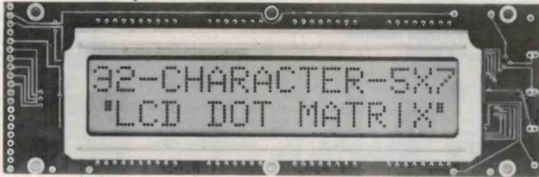
These intelligent dot matrix displays feature high contrast, wide viewing-angle and extremely low power drain. They feature 96 character ASCII set with internal ROM and LCD MUX drivers, and are ideal for microprocessor readouts.
