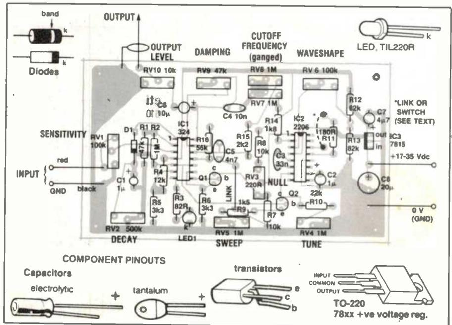
If you are using preset potentiometers for all the variable resistors, it is best to fit them all next. You may wish to use potentiometers, with knobs fitted, for RV2 and RV4 to 10. If so, leave these for the moment.
