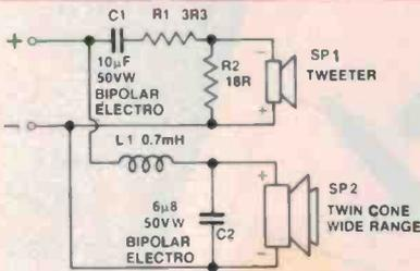
Circuit. Simple, isn't it. Note that the tweeter is connected in the opposite phase to the twin-cone to ensure their outputs add in the crossover region.
