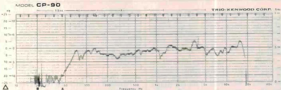
**Frequency response.** The speakers have a reasonably smooth frequency response (measured on the tweeter axis) with few significant peaks and dips. The bass response will lift somewhat when they're mounted near the floor.
