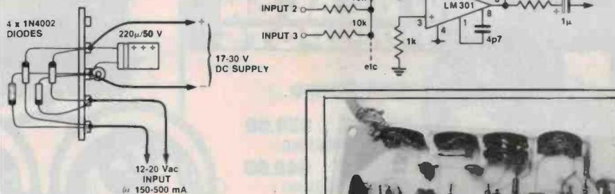
**Power supply.** Suggested construction details for a power supply. The ac input may be from a plugpack or ordinary transformer.
