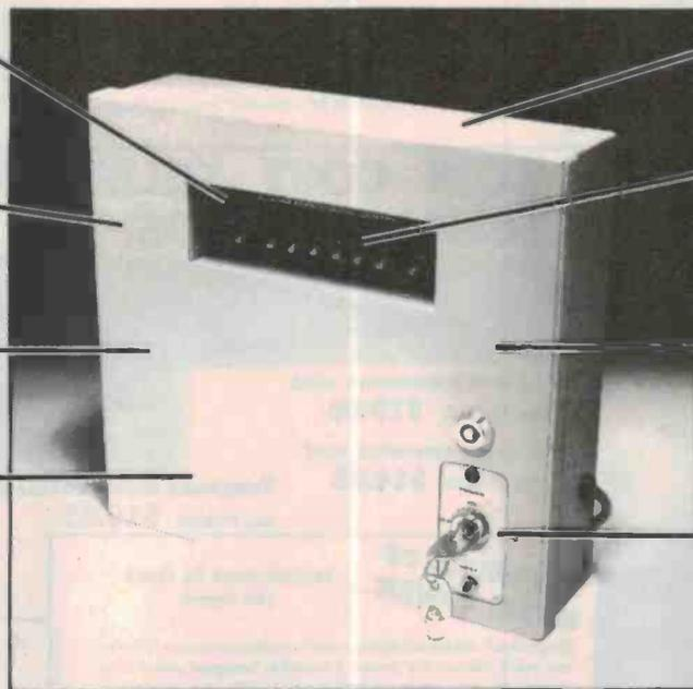
● Alarm circuitry is housed in high quality steel case fitted with anti-tamper switches.
