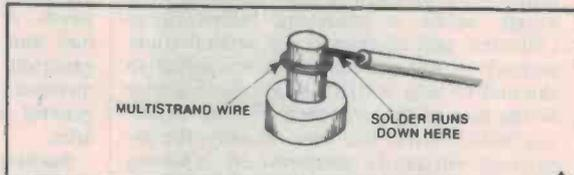
**Figure 19.** 'Wicking' is caused by solder running back up the strands of multi-strand hookup wire. This makes the wire brittle at the joint and movement may break it.
