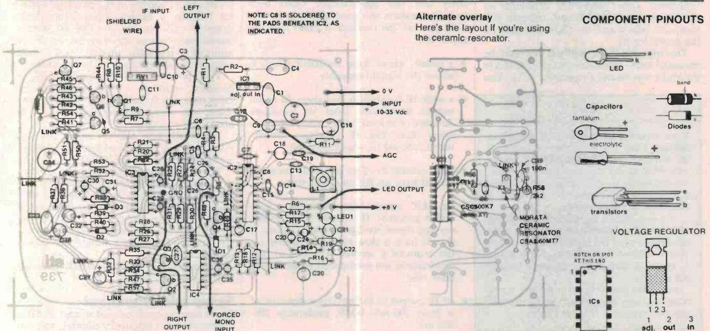
For effective stereo reception, the signal level here at the input needs to be above 150 mV RMS, which is generally easily obtainable in most good quality tuners or receivers. The decoder's input impedance is about 5k.
