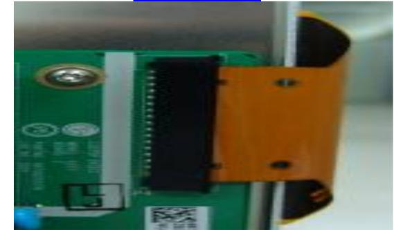
Connector to connect between Electrode PAD Of PANEL and Y Drive B/D,Z-Sus B/D
