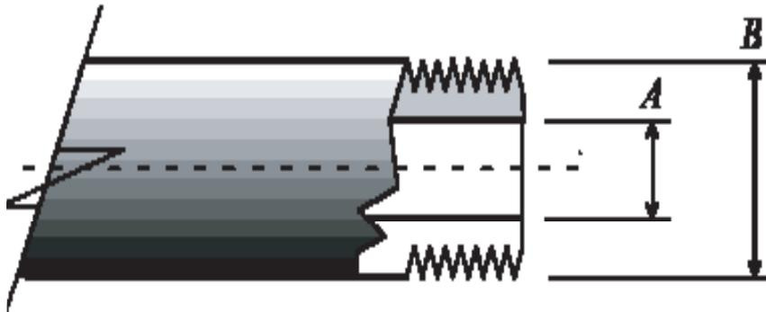
The industry designation for National Pipe Threads comes from the pipe's inside diameter (A). If you measure the outside diameter (B) of both the pipe or an actual sender with the same designation, it will be considerably larger than the NPT size.
