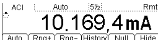
Figure 1- 15 AC Current Measurement Data Interface
